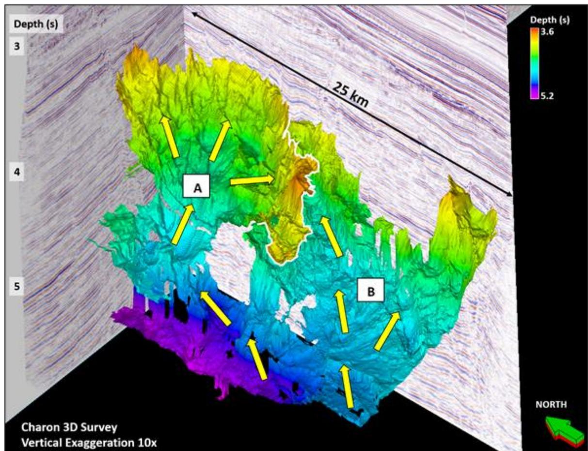
Figure 1. 3D interpretation of a magmatic plumbing system present in the Charon 3D seismic survey. Yellow arrows indicate direction of magma flow during emplacement of the intrusions.
