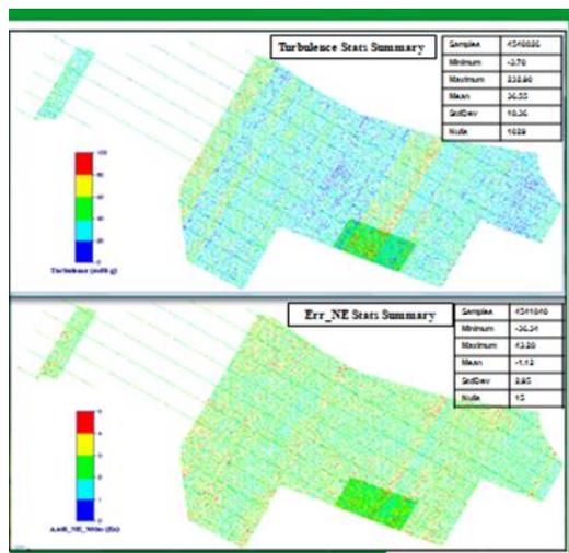
**Figure 1. Falcon Gravity Gradient field data from Brazil, in 2014 being subject to Quality Control check. A Frobenius Norm filter is used to check noise levels**
