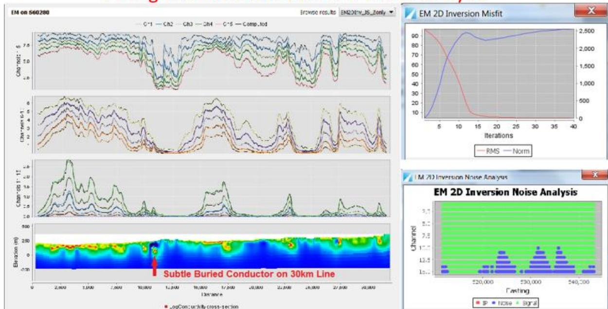
Figure 3. Use of 2.5D AEM inversion as a quality control checking tool. In South Australia, the Waddikee Tempest survey shows what portion of the measured signal is useable and what is below the noise floor.
