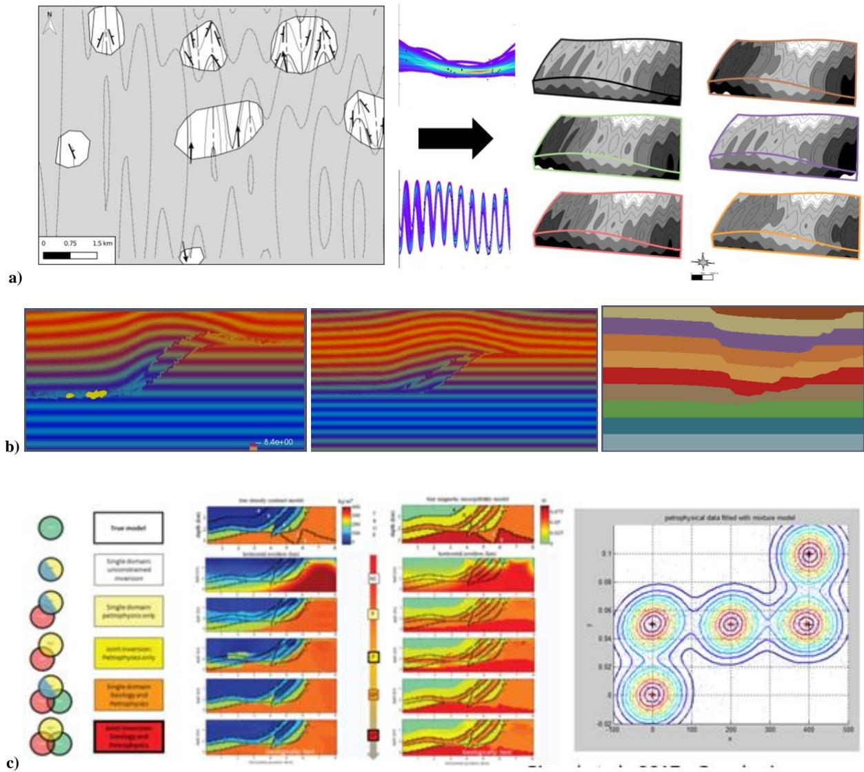
**Figure 2. a) Bayesian modelling of poly-folded stratigraphy; b) Bayesian modelling of faults and shear zones; c) geophysical inversion scheme utilising lithological probabilities.**
