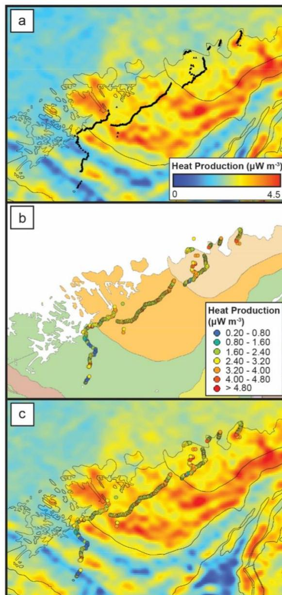
**Figure 2.** Results of heat production calculations from (a) calibrated airborne radiometric data (with ground-sourced measurement locations indicated by black triangles) and (b) ground-sourced measurements of U, Th and K (legend for lithological units is the same as Figure 1). (c) Comparison of heat production calculated from the separate datasets.
