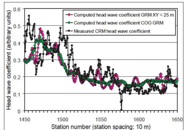
**Figure 1: Comparison of measured and computed head wave coefficients using P-wave seismic velocities computed with the traveltimes.**
