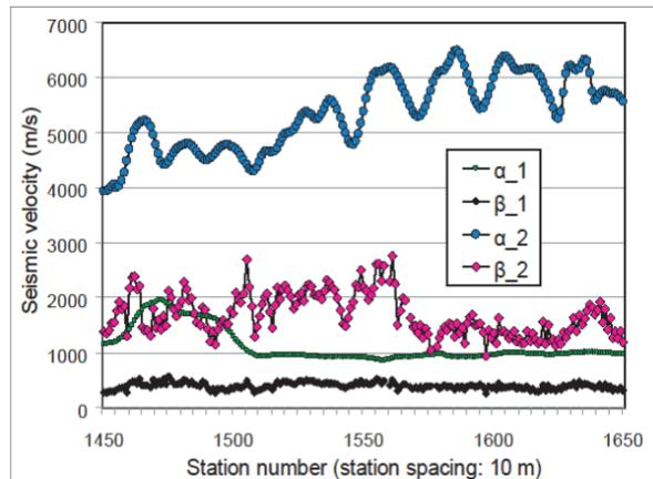
**Figure 6: Summary of P- and S-wave seismic velocities which reproduce the observed head wave coefficients in the weathered and sub-weathered regions.**
