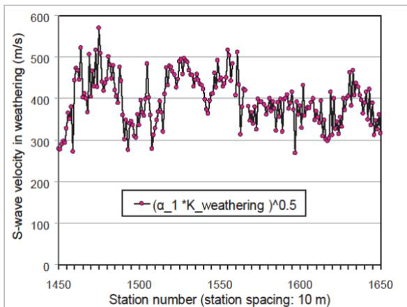
**Figure 4: S-wave velocity in the weathered layer computed with the P-wave velocity and the head wave coefficient in the weathered layer.**
