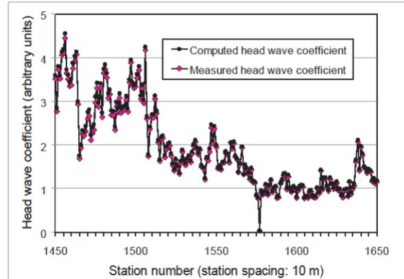
**Figure 5: Comparison of measured and computed head wave coefficients.**
