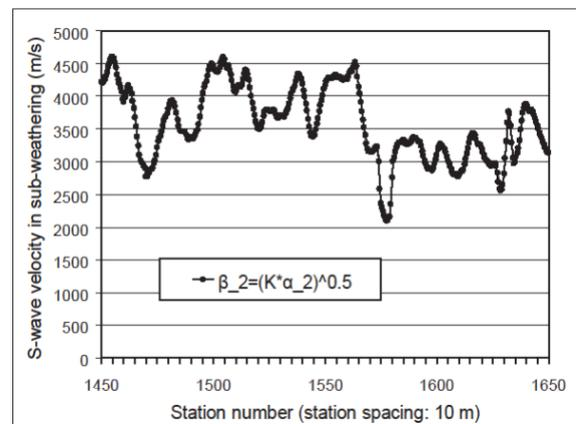
**Figure 2: S-wave velocity in the sub-weathered layer derived from the P-wave velocity and the head wave coefficient.**
