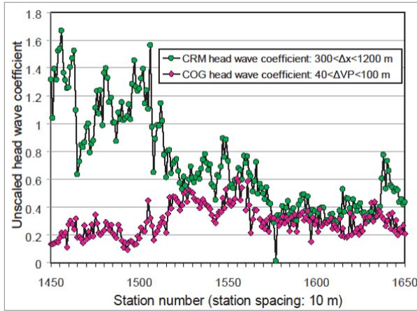
**Figure 3: Unscaled head wave coefficients computed with near and far trace offsets.**
