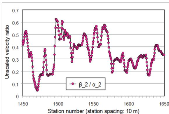
**Figure 7: Unscaled ratio of S- to P-wave seismic velocities in the sub-weathered region.**
