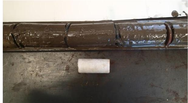
**Figure 4 – XL-Rock samples in the barrel compared with standard rotary side wall core.**
