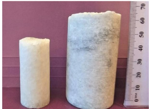
**Figure 1 – Standard rotary side-wall core sample (0.92”x 2”) compared with large rotary side-wall core sample (1.5” x 2.5”)**
