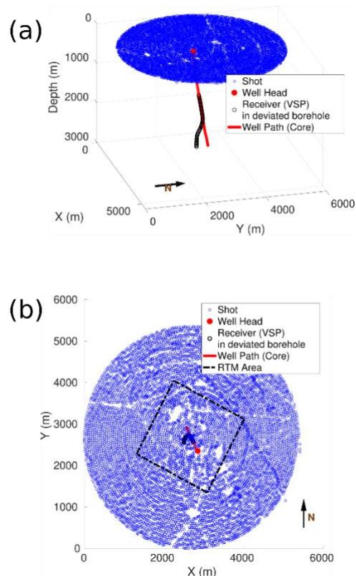
**Figure 1. 3D VSP acquisition geometry (a), and plan view (b). RTM area in (b) refers to reverse time migration.**
