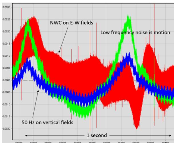
**Figure 1. A one second recording by the Loupe receiver in an urban area (Swanbourne), with transmitter turned off, shows the various noise contributions that need to be removed from final data.**
