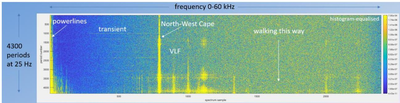
Figure 2. Spectra (DC – 60 kHz) of Loupe vertical component signals collected whilst walking, with the transmitter off, in an urban area. This is approximately 3 minutes of raw time-series (approximately 60 Mbytes in this case).
