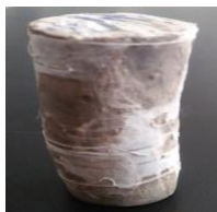
Figure 3. Shale core plug sample after spontaneous imbibition.
