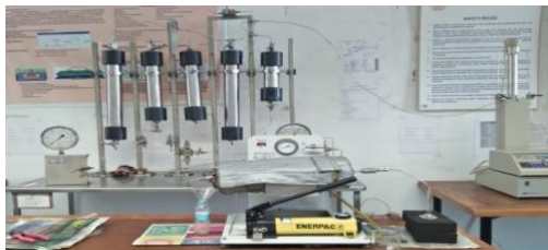
Figure 4. Core flooding system to establish permeability
