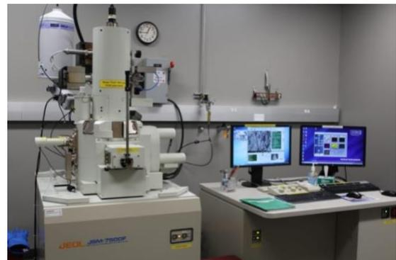
**Figure 1. Scanning Electron Microscopy (SEM) Instrument for taking Microscopy Images of shale sample.**
