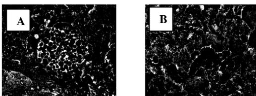
**Figure 3. Binarized the images by Image processing using threshold operation on (A) Jara and (B) Ratia samples.**
