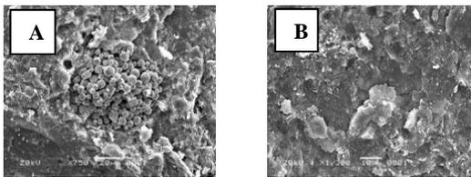
**Figure 2. The SEM Images of Shale from Jhuran formation of (A) Jara and (B) Ratia, Kachchh basin, 20x.**
