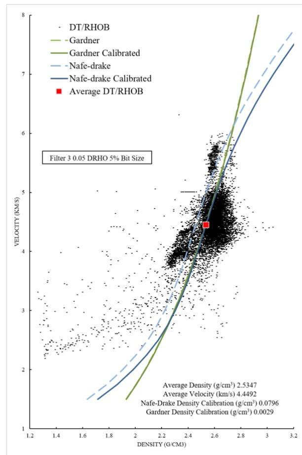
**FIGURE 1.** Cooper Basin regional velocity/density data filtered by 0.05 DRHO and 5% bit size. Overlaid are the Gardner and Nafe-Drake density sonic transforms and their calibration to the regional density/velocity average.
