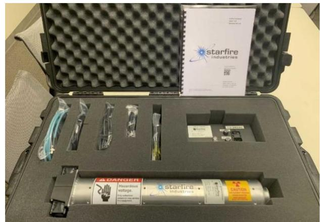
**Figure 1. nGen-310-DD neutron generator, powered by Starfire Industries nGen technology.**
