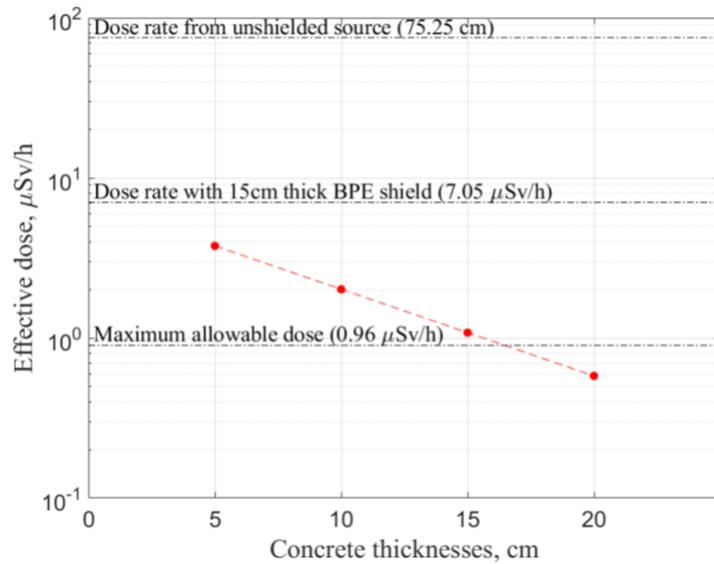
Figure 3. Effective dose rate obtained with shielding configuration with varying thicknesses of concrete.
