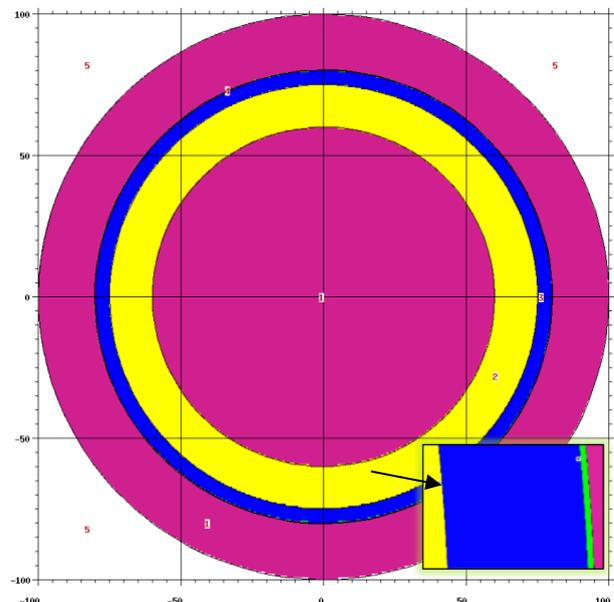
**Figure 2. Shielding model simulated in MCNP6.1. Air filled sphere with the shielding inside is represented in pink colour. Fixed 15 cm of BPE is yellow coloured; varying thicknesses of concrete (5 cm in this figure) is depicted blue. Being too thin (only 0.22 cm), Pb layer is represented in enlarged image area (green coloured).**
