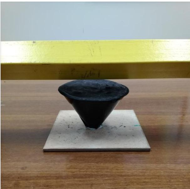
**Figure 1. The funnel model placed beneath the track along which the 3 component magnetometer travels.**
