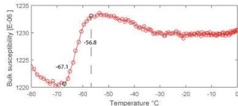
Figure 5. Close-up on suppressed Morin transition in one of a high grade hematite ore samples at Blötberget.
