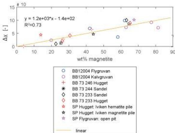
Figure 2. Plotted delta mass susceptibility at high temperature for magnetite (580 °C) transition and respective wt% magnetite. Samples are colour coded for drill core and ore body designation. Linear relation wt% and Curie temperature transitions below 600°C.
