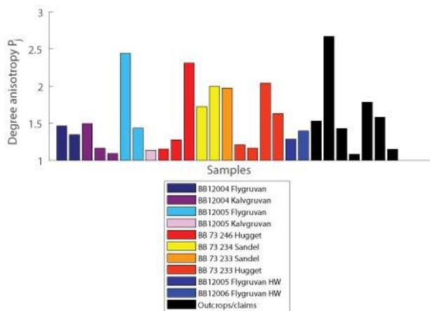
**Figure 6.** Measured degree of anisotropy ( $P_j$ ) for samples, colour themed for drill hole and ore body locality or outcrops/claims.
