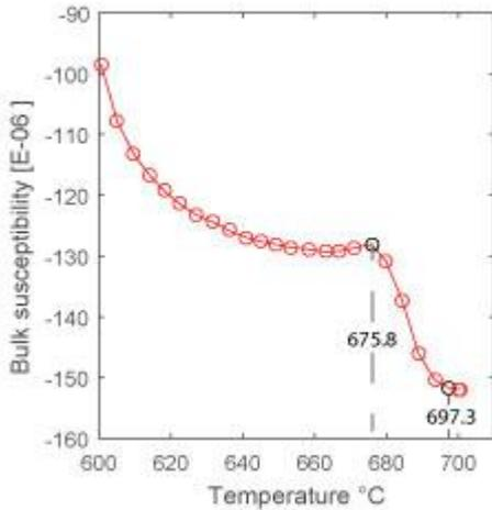
Figure 1. Measurement data from one of the 37 susceptibility temperature dependency sample tests. Curie temperature, approximately 580 °C, averaged at transition. The delta bulk susceptibility is difference between the same points in y-axis
