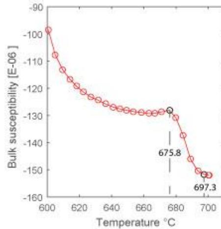
Figure 3. Measurement data for one of the ten samples where susceptibility temperature dependency sample tests. Néel temperature, approximately 680 °C, averaged at transition. The delta bulk susceptibility is difference between the same points in y-axis
