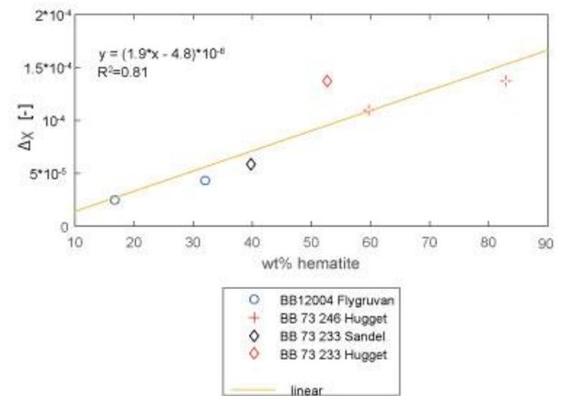
Figure 4. Plotted delta mass susceptibility at high temperature for hematite (680 °C) transition. Samples are colour coded for drill core and ore body designation. Linear relation between wt% and Néel temperature transitions between 600°C and 700°C.
