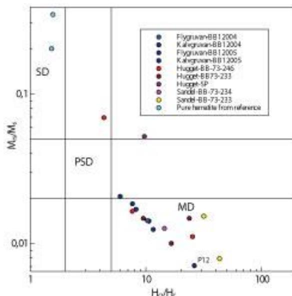
**Figure 7.** Magnetic hysteresis properties as function of wt% magnetite and locality. Day Plot in log scale with  $H_{cr}/H_c$  versus  $M_{rs}/M_s$ . Abbreviations SD ‘Single domain’, PSD ‘Pseudo single domain’ and MD ‘Multidomain’.
