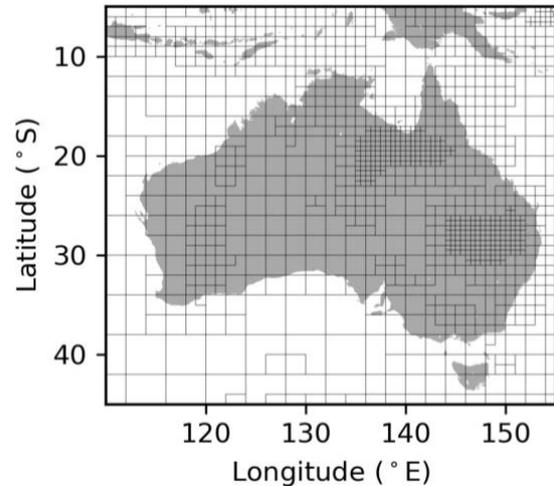
**Figure 2.** Example of an irregular grid-mesh used in tomographic modelling. Grid-size is adapted to the current model resolution.
