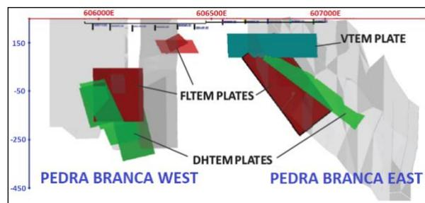
**Figure 5. Long Section of the Pedra Branca deposits (grey surface) showing the improved spatial resolution provided by the FLTEM and DHTEM modelling, over the VTEM modelling**
