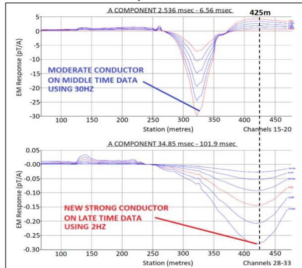
**Figure 4. DHTEM data comparison of historic 30Hz survey (top) and more recent 2Hz survey (bottom) showing the associated new late time anomaly at 425m**
