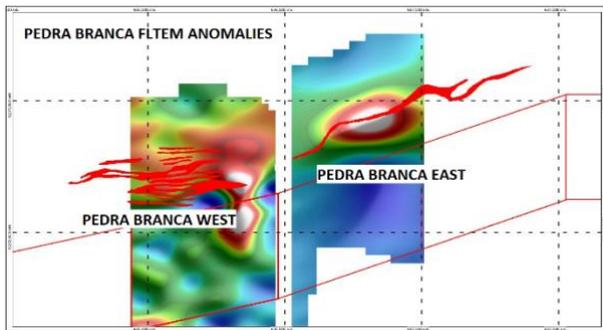
**Figure 2. Fixed Loop TEM surveys over Pedra Branca deposits. Image is of B-field X component (6.093 msec). Mineralisation is in red and loops are shown as thin red lines**
