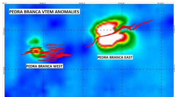
**Figure 1. Airborne electromagnetic survey (VTEM) image (0.3 msec) over the Pedra Branca deposits (mineralisation in red)**
