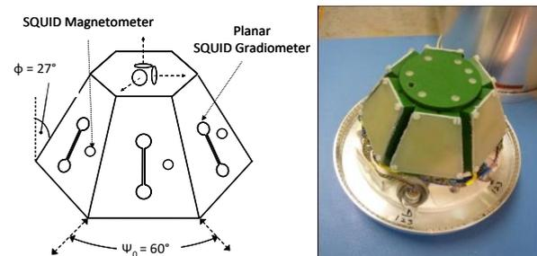
**Figure 9. Schematic (left) and photo (right) of the full tensor magnetic gradiometer which uses six planar SQUID gradiometers with multiple reference sensors.**
