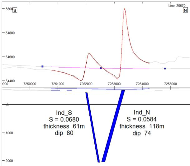
Figure 4. Best-fit induced magnetization model for line 20670 (location shown in Figures 2 and 3).
