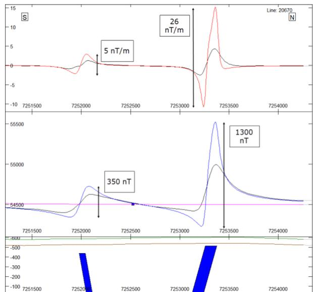
Figure 7. Magnetization directions of the north and south fold limbs for the steeper and shallower dip models.
