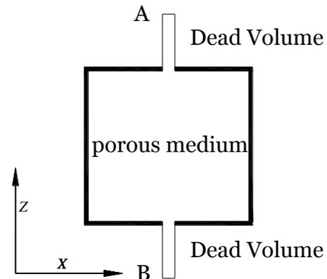
**Figure 1. The model of the porous medium with dead volumes**
