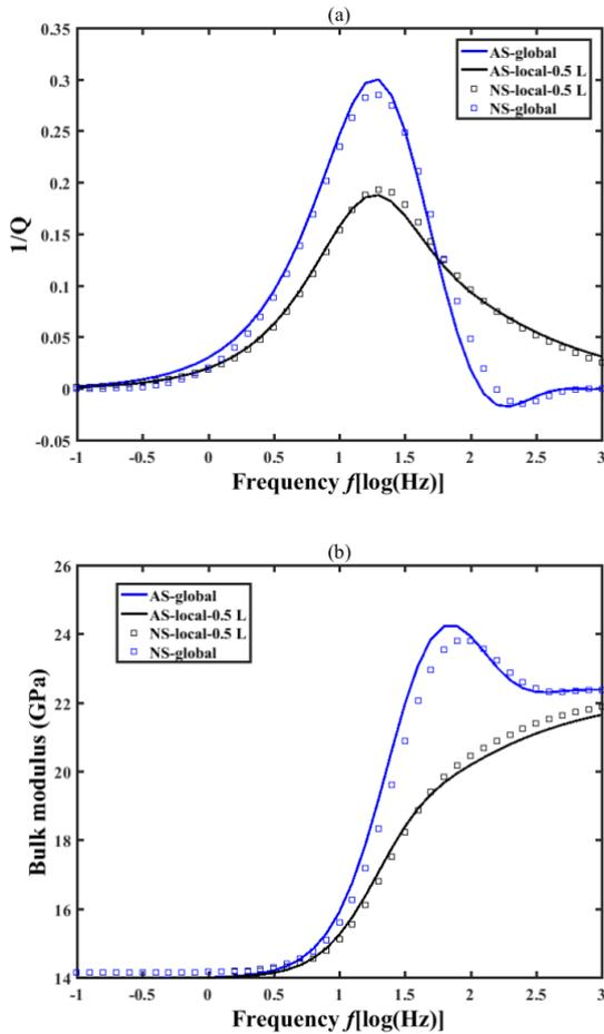
Figure 2. The attenuation (a) and the real part of Young’s modulus (b) obtained from the numerical (NS) and
