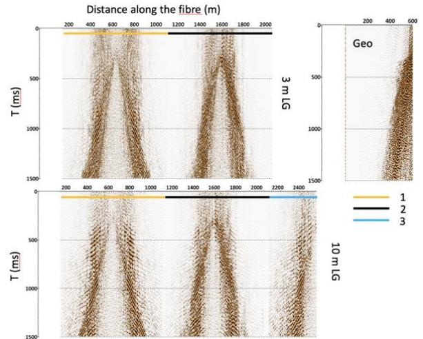
Fig. 3. Raw data example for geophone and 3 m gauge length (10) and 10 m gauge length DAS units. Note that fibre forms one continuous line comprised of tactical (1), telecom (2) and bare fibre (3, for 10 LG unit only). The shot is at the end of the line.
