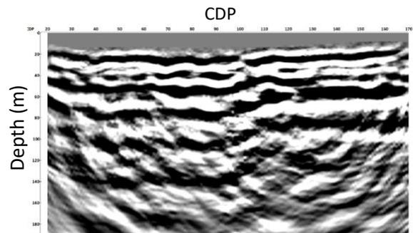
Fig 4. The pre-stack depth migration with a TMDDF filter, which adds a great improvement and enhances the quality of the final imaging.
