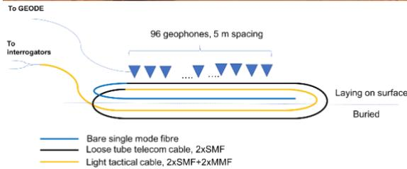
Fig. 2. Cable and geophone layout scheme. Two systems of a conventional seismic line and DAS cables are shown in the figure. Also shown is the conventional seismic line (gray arrow) with 96 channels. DAS cables are buried into different places to cover most of the study area.
