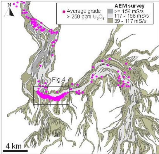
**Fig. 2.** Geological map of the Yarramba paleochannel interpreted from TEMPEST™ airborne electro-magnetic (AEM) survey results (BOSS Resources, unpublished data). Different colours denote lithofacies. Dots denote the drillholes intersecting uranium mineralisation.
