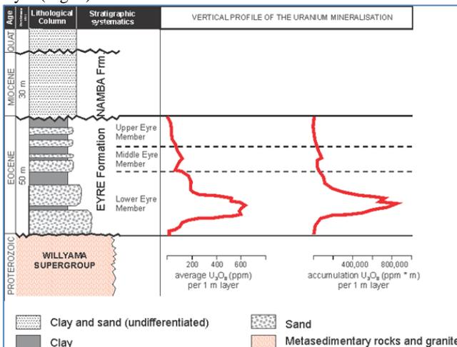
**Fig. 3.** Stratigraphic column of the Yarramba paleochannel and vertical profile of the uranium mineralisation (based on 1689 drillholes).
