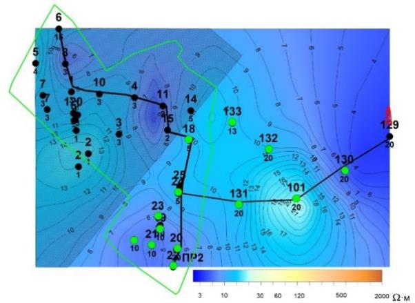
**Figure 5. TEM resistivity map to the depth of 40m**
