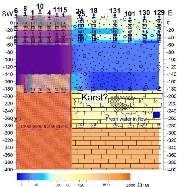
**Figure 4. TEM geoelectric section**
