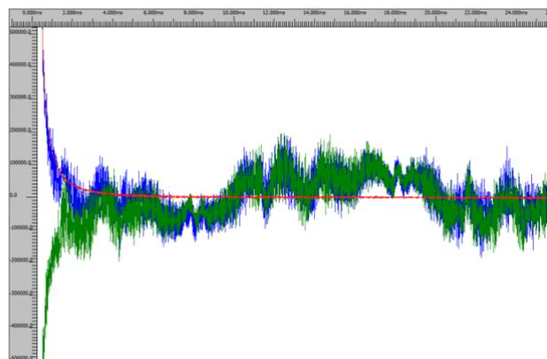
Figure 3. The initial EMF decay (negative and positive polarity are green and blue graphs, respectively) complicated by a 50 Hz power lines interference and the result of digital interference processing (red graph).
