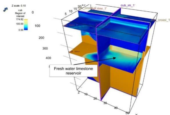
**Figure 6.** 3D TEM resistivity model
