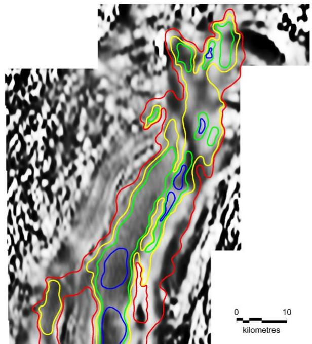
Figure 3. Depth contours derived from the Naudy analysis of the Kilombero aeromagnetic data, over RTP1VD image. Red = 1km, Yellow = 2km, Green = 3km, Blue = 4km.
