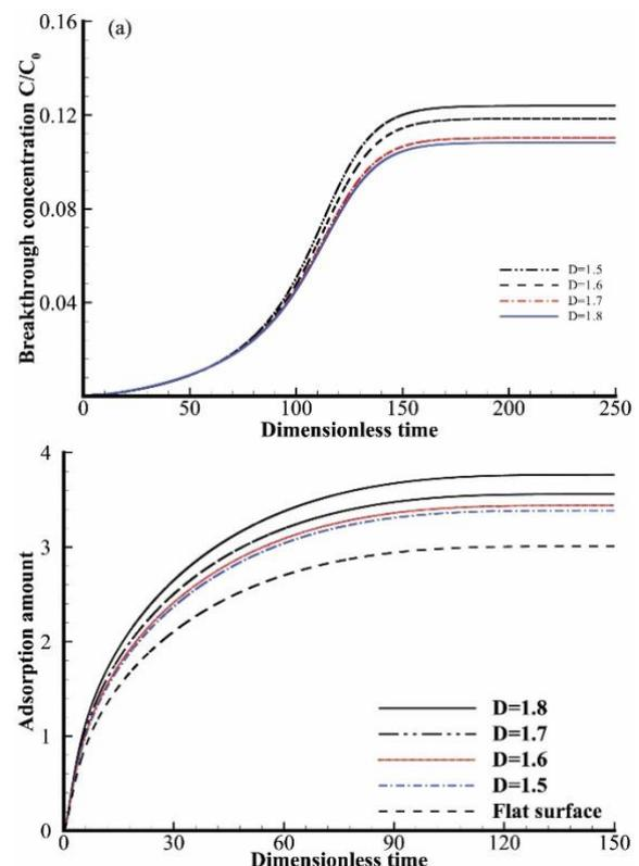
**Figure 2.** Partial results of investigations of the methane transport in a rough cleat for various  $D$ . (a) Breakthrough curves; (b) Adsorption curve.
