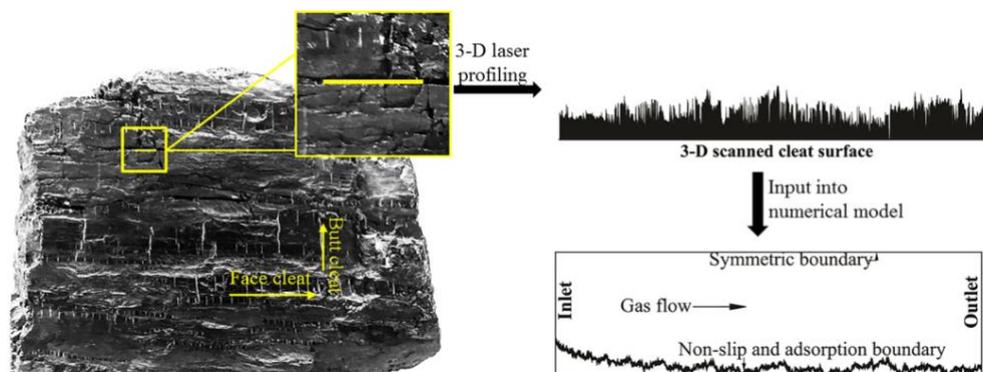
Figure 1. Procedures of 3-D image analysis and construction of a numerical model based on the scanned rough cleat surface.
