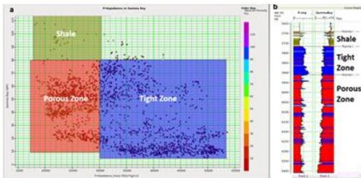
**Figure 1. (a)Cross-plot of P-impedance Vs Gamma Ray The x-axis is P-Impedance and the y-axis is Gamma Ray.(b) Attribute cross section P-Impedance Vs GR cross-plot for T Well. It shows the tight zone, porous zone and shale**
