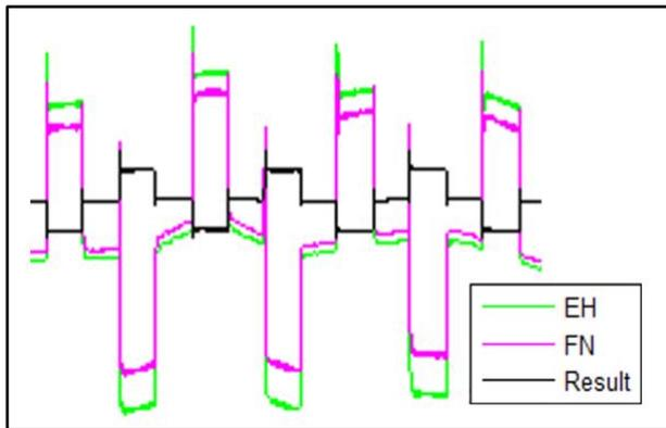
**Figure 1: Example of the subtraction of the time series response from two electrode sensors, EH and FN. Sample Rate = 150 sps.**
