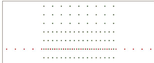
**Figure 4: Rolling 3D survey layout: survey lines are horizontal, red dots are current injection points, green dots are receiver electrodes. The receiver electrode array relative to the current injections is maintained as the current injection progress from line to line to complete the survey**
