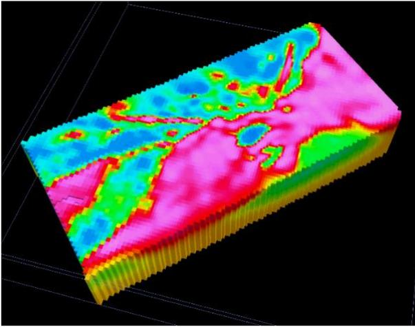
**Figure 5b: 3D inversion result based on the pole-dipole data set showing an elevation plan at a depth of approximately 50 m – blue is resistive.**
