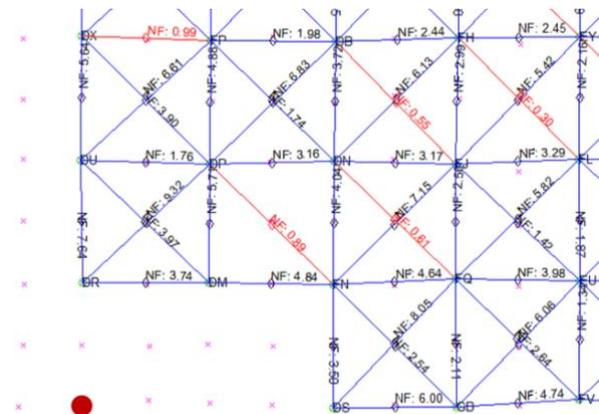
**Figure 3: Plan view of part of the dipole building process for a 3D CVR survey. Receivers are located at each of the nodes. Rejected dipoles are red; accepted dipoles are blue, and the current input is the red dot.**
