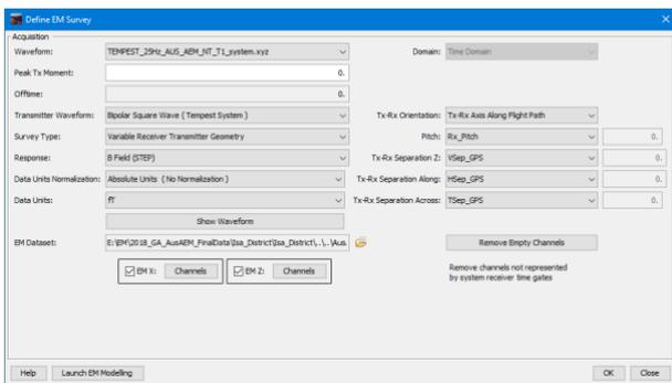
**Figure 2. 2.5D Inversion set-up window showing incorporation of variable receiver-transmitter geometry**
