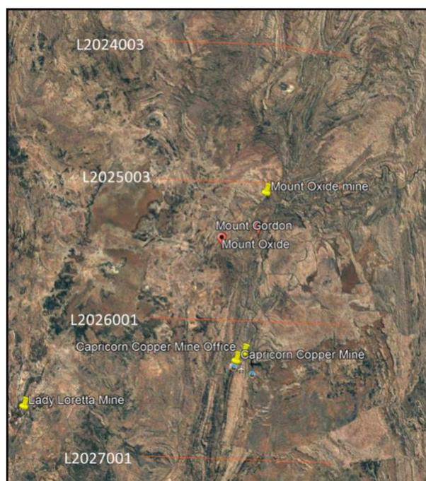
**Figure 5.** Extracts of AusAEM TEMPEST survey lines in the vicinity of the Capricorn Copper and Mount Oxide Mines, shown on Google Earth imagery. Survey lines spaced at 20km.
