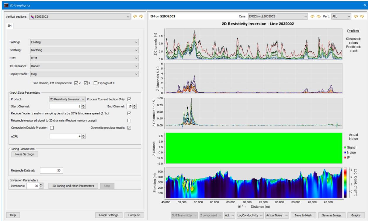
**Figure 3.** Example of the Moksha 2.5D inversion GUI inside GeoModeller. Conductive stratigraphy associated with the Mount Isa orebody is evident near the western (left) end of the line.
