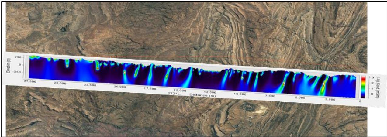
Figure 8. 2.5D inversion section of log conductivity from the Mammoth Mines area, showing steeply-dipping conductors and possible exploration targets. The folded surface geology can be directly translated to anticlinal or synclinal features, with conductive marker beds indicating the near surface fold limb dips.
