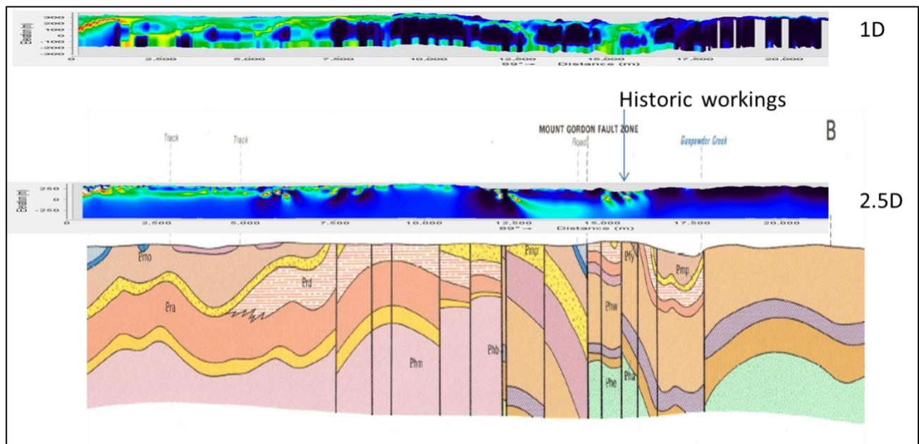
**Figure 7.** Results of 1D and 2.5D inversions from Line 2026001 over the Mount Gordon Fault Zone. Images are of log conductivity. The 2.5D inversion result shows clearly defined moderate to steeply-dipping conductors associated with the
