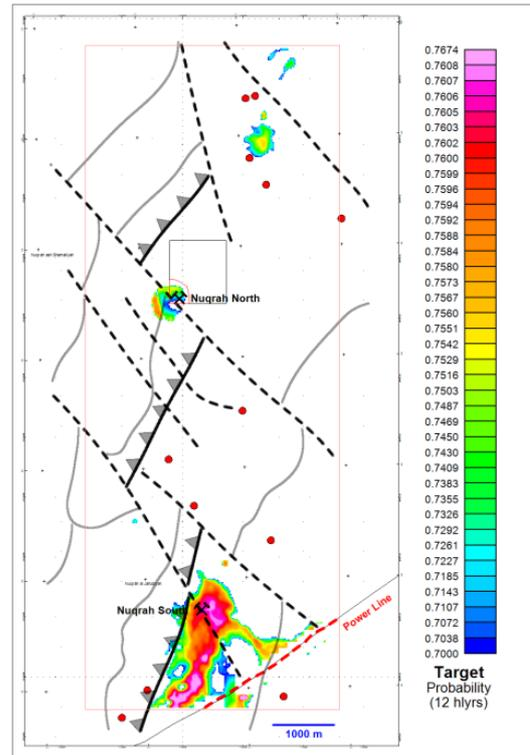
**Figure 8.** Top 90% target probabilities generated from a DNN with twelve hidden layers.
