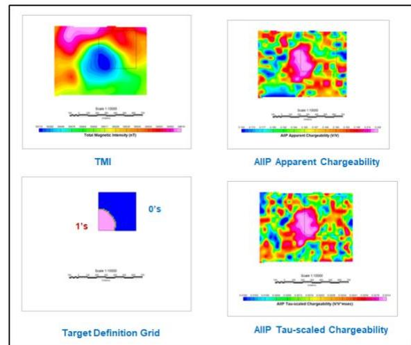
**Figure 4. TMI, AIP apparent chargeability, AIP TSC test data, and target definition grids over a known kimberlite in the Canadian Shield.**
