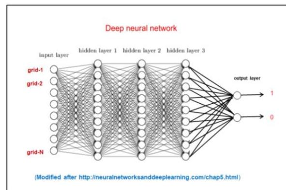
Figure 2. A simple three hidden layers DNN with two output classes, 1 and 0.
