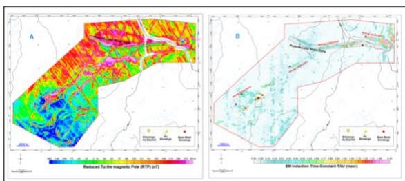
Figure 10. (A) Reduced-to-pole (RTP) data and (B) EM induction time-constant data of the Kabinakagami Lake TDEM survey area.
