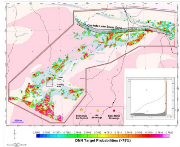
Figure 12. DNN top 75% predictive targeting probabilities for possible Au mineralisation in the of the Kabinakagami Lake TDEM survey area. The final DNN results are masked using the KLGB outline polygons.
