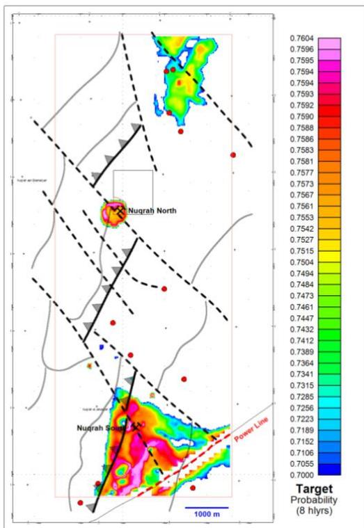
**Figure 7.** Top 70% target probabilities generated from a DNN with eight hidden layers; red dots indicate known SEDEX occurrences.
