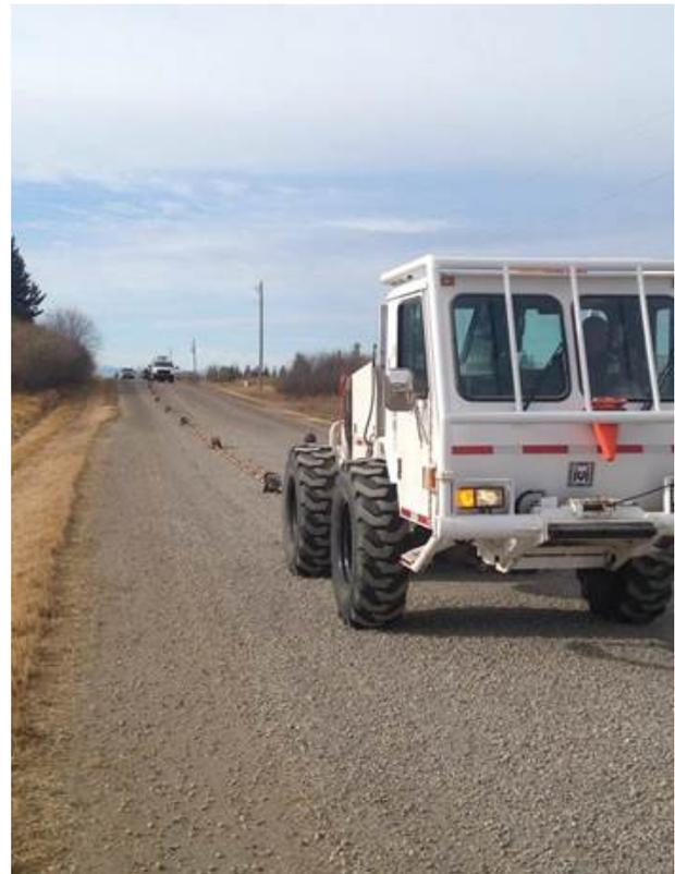
**Figure 1. Survey in progress. Envirovibe with land-streamer in tow.**
