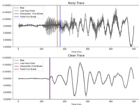
**Figure 1.** Example of seismic refraction traces from the dataset in use. Note the high frequency noise appears in multiple temporally discrete segments. A low-pass filter has been applied to each trace. There are also the first break picks of each trace. One noted mid acquisition (field) the other chosen in post processing (interpreter).
