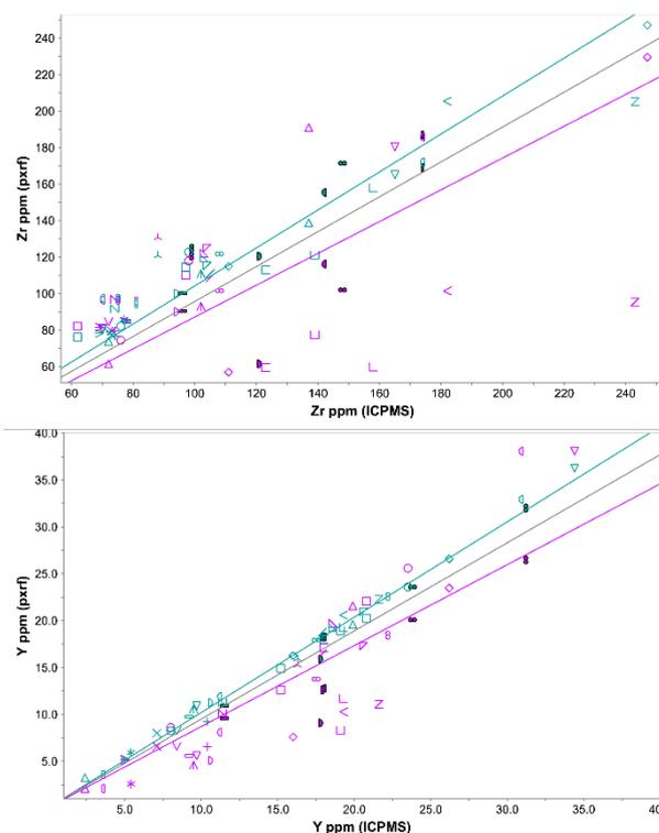
Figure 2. Comparison of pXRF and ICPMS data for Zr and Y. Blue points are pulp analyses, purple are rock analyses. Grey line is regression of all data. Point shapes represent different samples.
