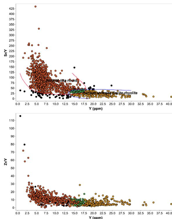
Figure 1. Sr/Y vs. Y and Zr/Y vs. Y plots of global porphyry data. Colours represent prospective (orange) mixed (green) and un-prospective (yellow) fields in Sr/Y vs Y plot.
