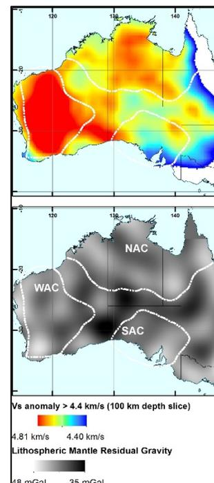
**Figure 1. Top; Shear wave velocity 100 km depth slice from AuSREM (Kennett et al., 2013). Bottom; Wavelength-filtered gravity anomaly map (after Sandwell et al., 2014) showing variations beneath the crust. White dashed lines represent the approximate location of the North, South and West Australian Cratonic regions (NAC, SAC and WAC).**
