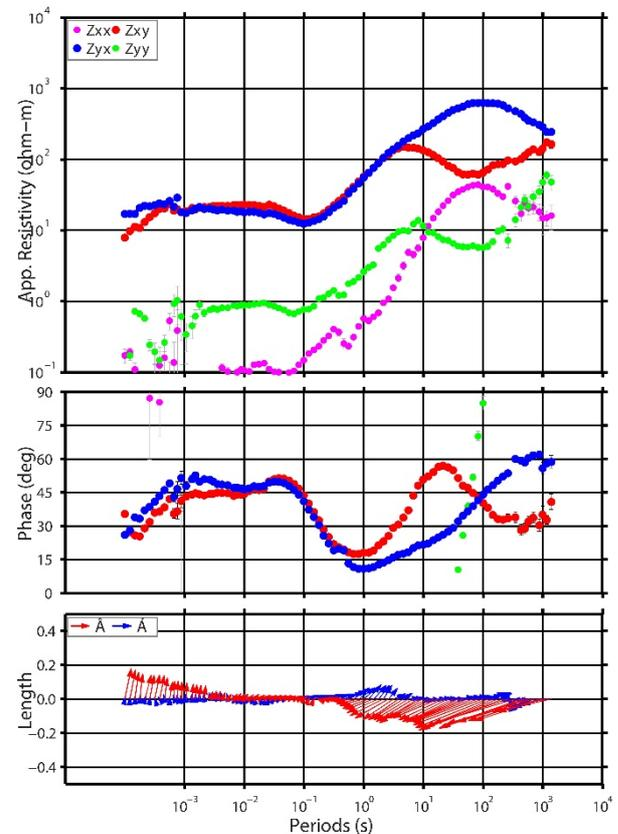
**Figure 2. Apparent resistivity (top), phase (middle) and induction arrow (bottom) plots of site 109 showing an example of the data quality.**
