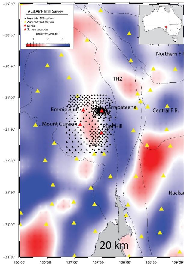
**Figure 1. Outline of the broadband and audio-magnetotelluric stations (black triangles) of the new Olympic Domain in-fill survey on top of a 20 km depth slice of the 3D AusLAMP MT model across the Gawler Craton. Yellow triangles denote locations of the AusLAMP MT sites. The survey area is placed atop an elongated crustal conductor of the eastern Gawler Craton IOCG terrane. This survey is designed to provide an enhanced 3D resolution of this mineral system.**
