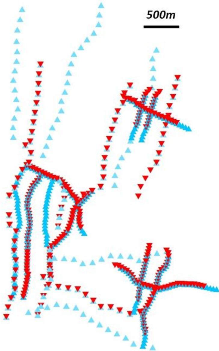
Figure 3. Plan view of customised irregular trilinear 3DIP array layout with electrode locations (blue = Rx, red = Tx).
