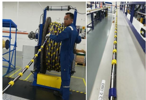
**Figure 2. Construction of test cable sections in manufacturing facility**
