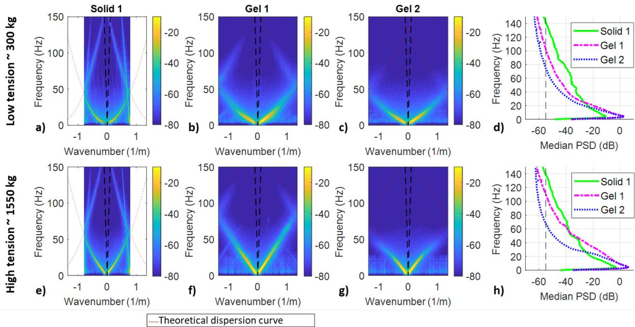
Figure 3. Frequency-wavenumber ( $f-k$ ) spectra of three different sections. Under low tension of approximately 300kg, a) – c) and their respective median power spectral densities (PSD's), d). Corresponding  $f-k$  spectra under high tension (1500kg), e) – g) and their median PSD's, h).
