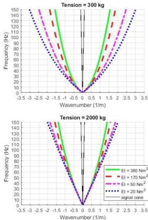
**Figure 1. Frequency-wavenumber ( $f-k$ ) dispersion curves for two plastic streamers (green and red) and two gel filled streamers (magenta and blue). The upper picture is for a low-tension case and the lower for high-tension.**
