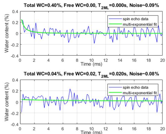
**Figure 5. Corona results for sample 786B\_S1, as-received sample showing impact of noise on inversion. Top: spin-echo decay data from 200 repeat scans of Test 1. Bottom: spin-echo decay data from 200 repeat scans of Test 2.**
