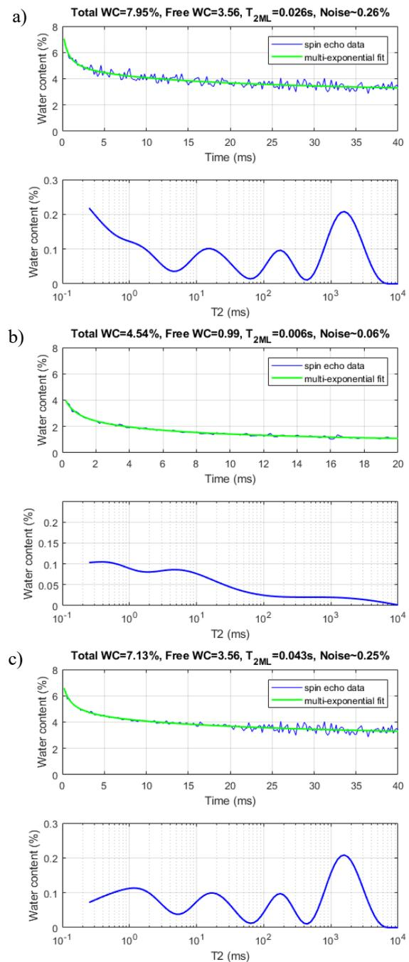
**Figure 6. Corona spin-echo decay data and T2 inversions from sample 784B for: a) 100 scans, 2s decay; b) for 2000 scans of 0.02s decay; and c) combined. Both a) and c) are truncated to 40ms for comparison. The short scan and polarization time leads to partial polarization and lower free water response, but provides significant improvement in SNR.**
