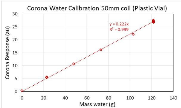
**Figure 2. Calibration of Corona showing good linear response to mass of water present.**
