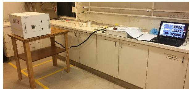
**Figure 1. Arrangement of Corona, control unit and laptop for testing blast hole chip samples.**
