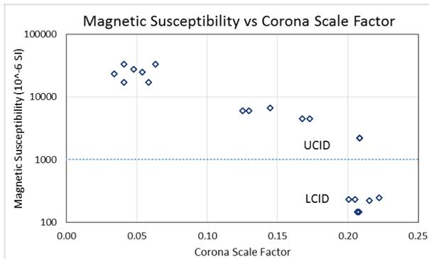
**Figure 7. Corona scale factor for a range of samples having different magnetic susceptibilities.**
