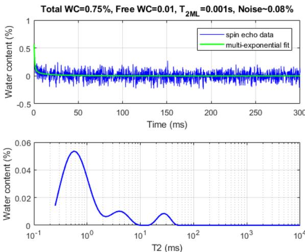
**Figure 3. Corona results for sample 786B\_S1, 9g water added; the twin dried sample indicated ~4g of water was present in the as-received sample. Top: spin-echo decay data from 200 repeat scans. Bottom: Inversion of data into T2 domain.**
