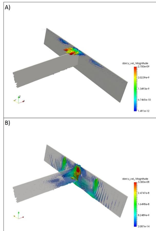
**Figure 4. Results of numerical simulations where Emu Fault has low permeability in the top 300m. a) Fluid flow within the BCF showing significant infiltration. b) Fluid flow within faults only.**
