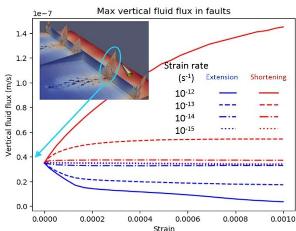
**Figure 5. Effect of deformation on convection: Maximum vertical fluid flux in the faults as a function of strain rate.**
