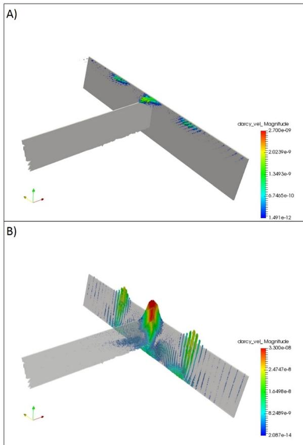
**Figure 3. Results of numerical simulations where Emu Fault has constant high permeability. a) Fluid flow within the BCF showing minor infiltration (contrast with Fig. 4a). b) Fluid flow within faults only.**
