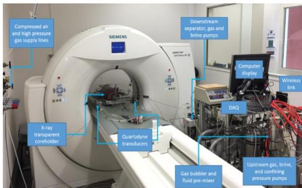
**Figure 3. CSIRO X-ray CT monitored core flooding rig.**
