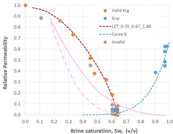
**Figure 4.** Gas relative permeability (orange dots are valid points) and brine relative permeability (blue dots). The red dashed line is the LET function fit. In pink is a default Corey function (solid- imbibition, dash- drainage).
