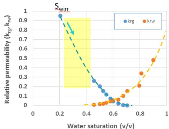
**Figure 2.** Example of a good quality, but incomplete imbibition relative permeability curve. There is a large data gap (yellow) in the gas relperm data between the gas-only flow point at  $S_{w,irr}$  and the first co-current flow point at  $S_w=0.43$ . Data from Maloney et al. (1994).
