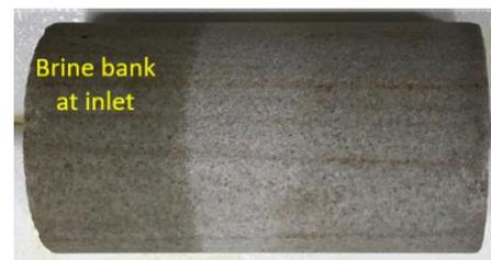
**Figure 1.** Berea sandstone sample taken from test rig at the early stage of an imbibition relperm measurement using existing SCAL methods. A large brine bank has formed at the inlet that blocks the permeability to gas.
