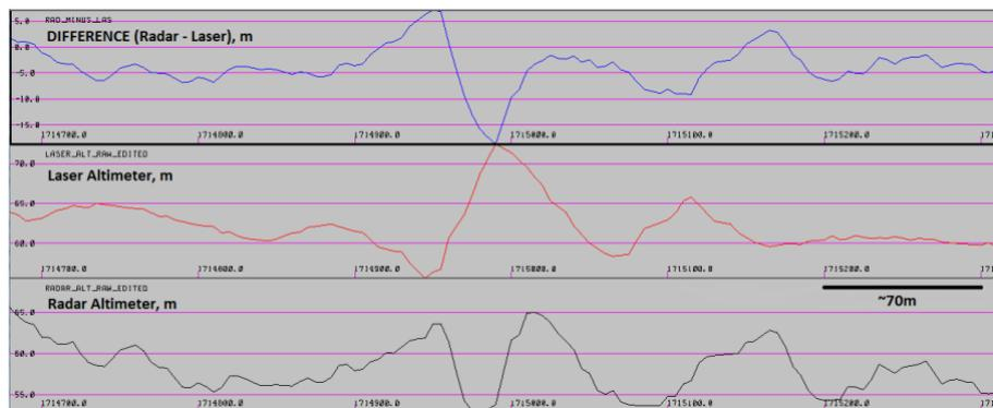
**Figure 1. Radar altimeter versus Laser altimeter responses in locally varying terrain. The responses are locally different by >10 m.**
