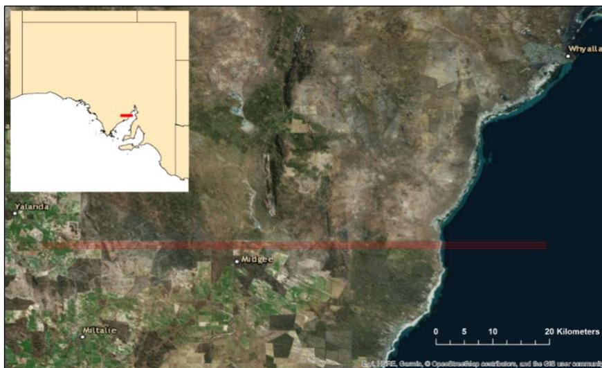
Figure 3. The location of the Whyalla Test Lines. There are seven E-W lines spaced 200 m apart. The lines are ~75 km long with the eastern portion extending over the Spencer Gulf.
