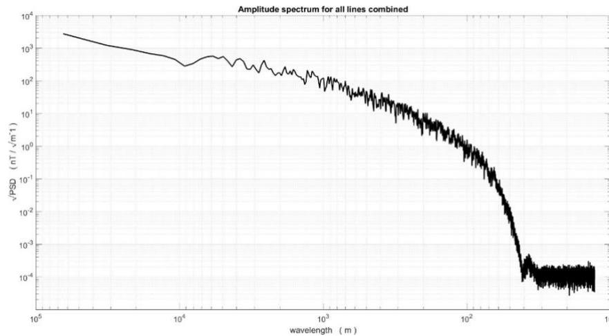
Figure 2. Amplitude spectrum of a single long line of raw magnetic data collected using one of the systems employed on GCAS. The sharp drop of the curve at ~50 m and subsequent ‘bounce’ are indicative of filtering of wavelengths <50 m.
