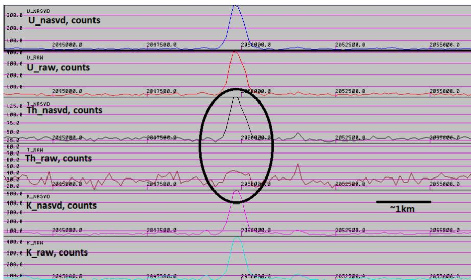
Figure 4. Profiles of raw and NASVD adjusted radioelement window counts from a line of GCAS data: from top to bottom, Uranium (U) NASVD, U raw, Thorium (Th) NASVD, Th raw, Potassium (K) NASVD and K raw. An example of a false Thorium (Th) anomaly generated by the application of NASVD can be seen within the black ellipse. False Th anomalies were generated when a strong U anomaly was measured in the absence of a strong coincident Th anomaly.
