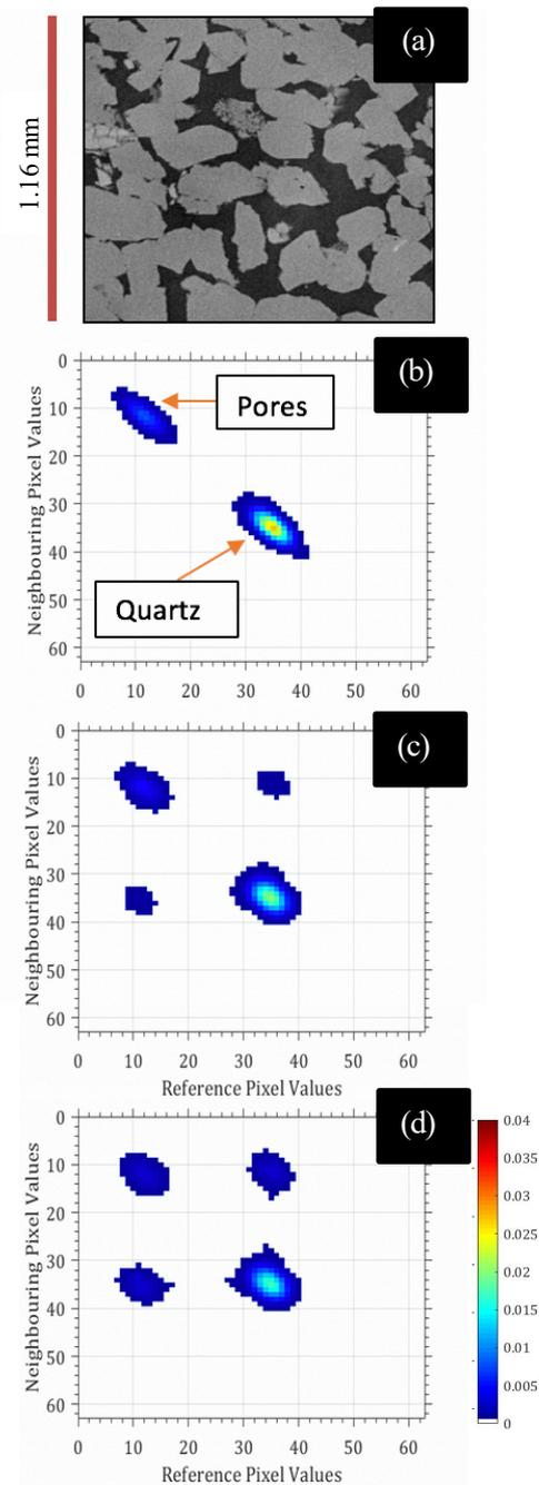
**Figure 1. GLCM map for the Bentheimer sandstone. (a) A  $400 \times 400$  2-D Slice of a Bentheimer sandstone with a resolution of  $2.92 \mu\text{m}$ . This image is re-quantized to a 6-bit image, (b) GLCM map of Bentheimer sandstone in (a) using an orientation of  $0^\circ$  with displacement vector of 1, (c) GLCM map using a displacement vector of 7, and (d) GLCM map using a displacement vector of 15.**
