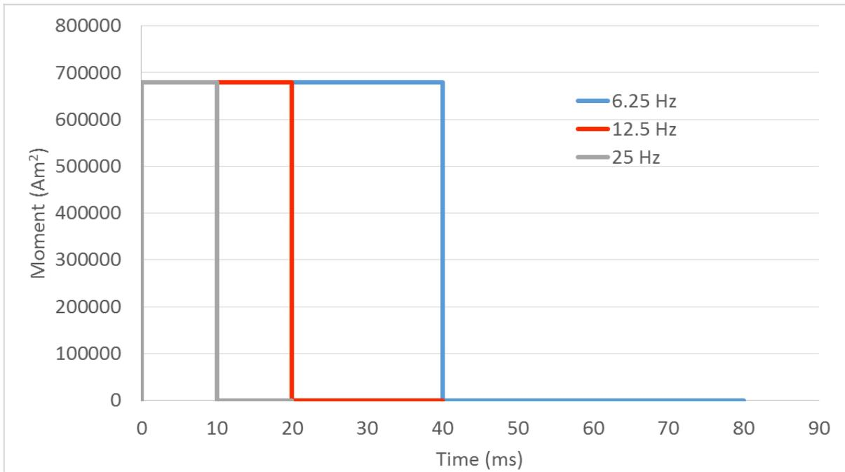
Figure 1. 50% duty cycle waveforms for at 25, 12.5 and 6.25 Hz.
