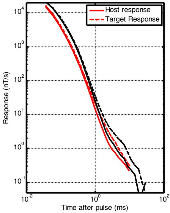
Figure 5. Measured transient decay from the 6 ms half-sine waveform (red) and 7.5 Hz 33.3 ms square waveform (black) above the 300 S target (dashed lines) at position 1,700 m in Figure 4 and the background response (solid lines) at position 1,400 m.
