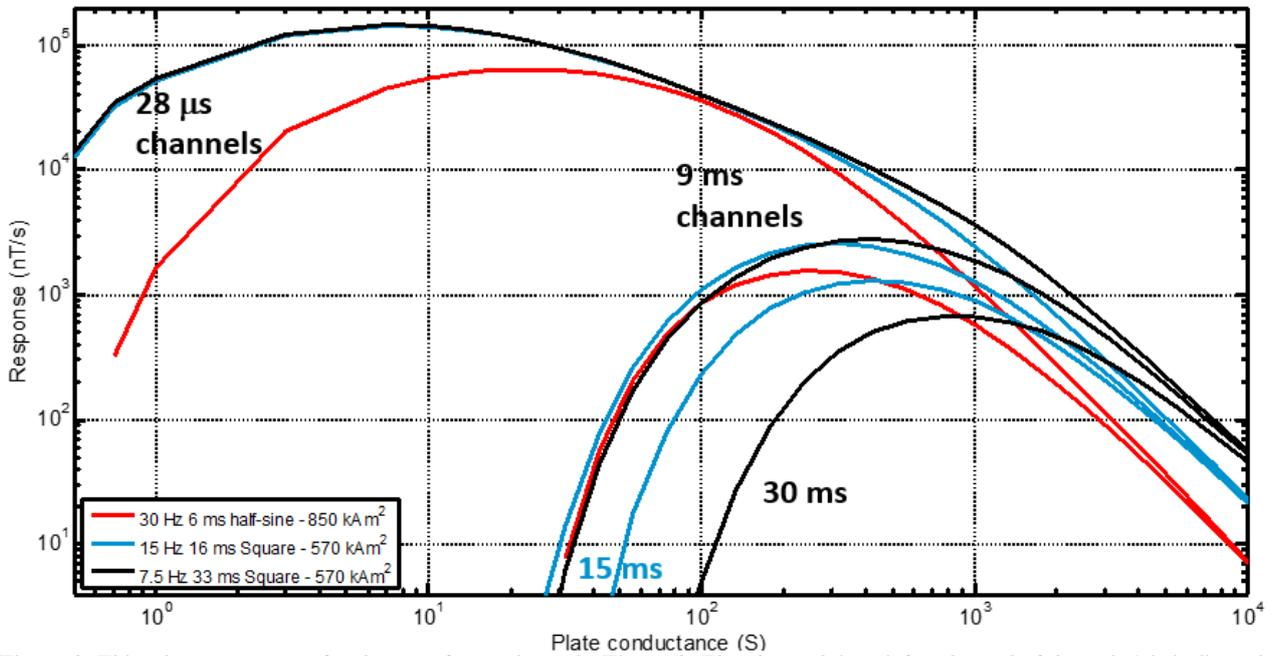
Figure 3. Thin plate nomogram for the waveforms shown in Figure 2. The channel time (after the end of the pulse) is indicated. The 15 Hz and 7.5 Hz waveforms have a longer off-time and their last channel has been plotted as well.
