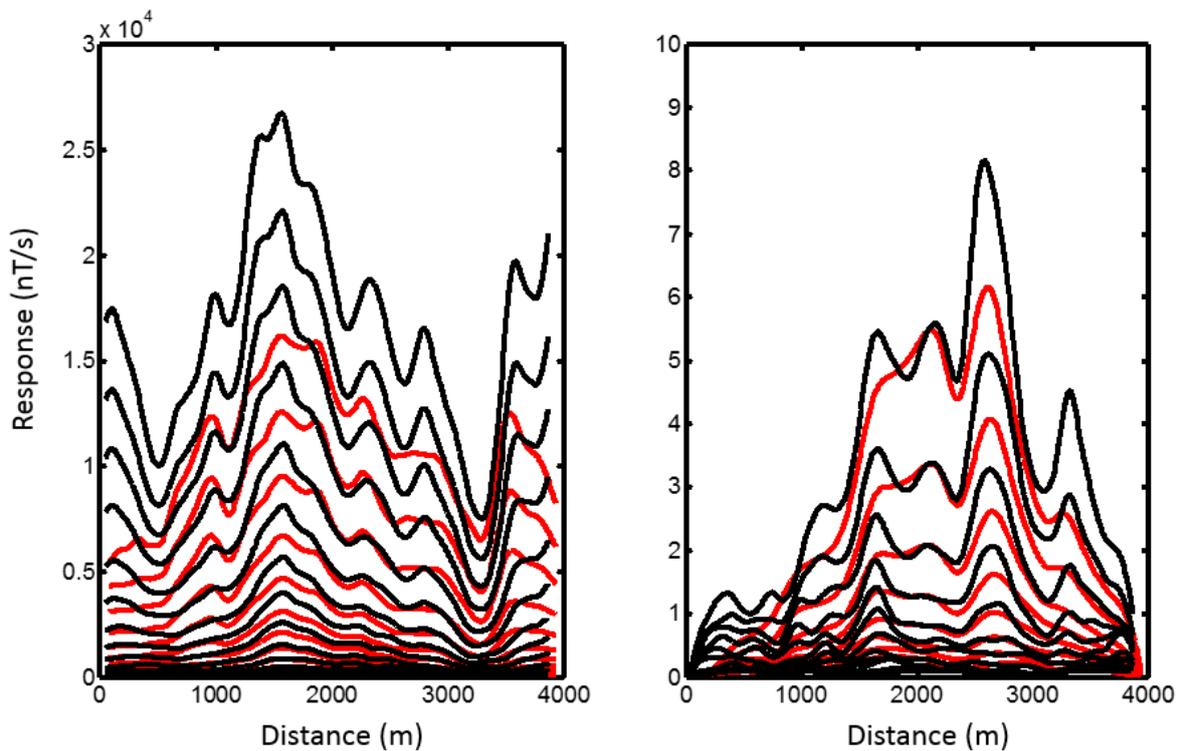
Figure 4. Measured response from the 6 ms half-sine (red) and 7.5 Hz square-wave (black). Left side shows early-time channels. Right side image shows late-time channels (from 3 ms after the end of the pulse).
