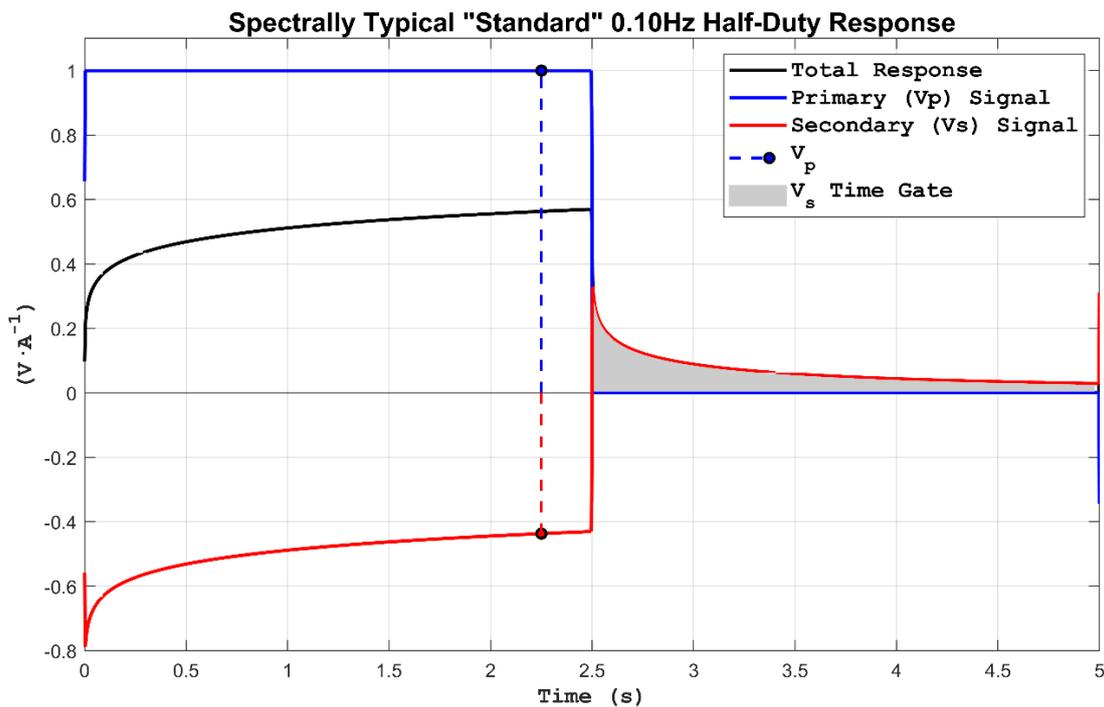
**Figure 1.** Primary and secondary signals comprising a total response are illustrated in terms of a spectrally typical Cole-Cole theoretical model ( $\tau = 1.0, c = 0.225$ ). The total response (black curve) during the off-time or decay is masked by the secondary response curve as, during the off-time, the two are identical.
