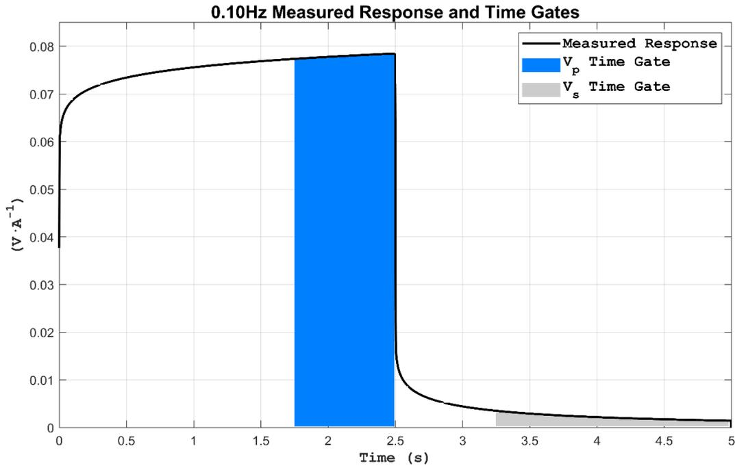
Figure 2. A hypothetical measured response is shown, along with hypothetical time gates employed to estimate, as a time-gate average, primary ( $V_p$ ) and secondary ( $V_s$ ) signals.
