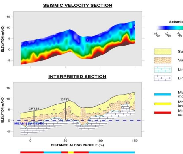
**Figure 2. p-wave and interpreted models of dune structure perpendicular and adjacent to beach with CPT refusal depths overlaid.**
