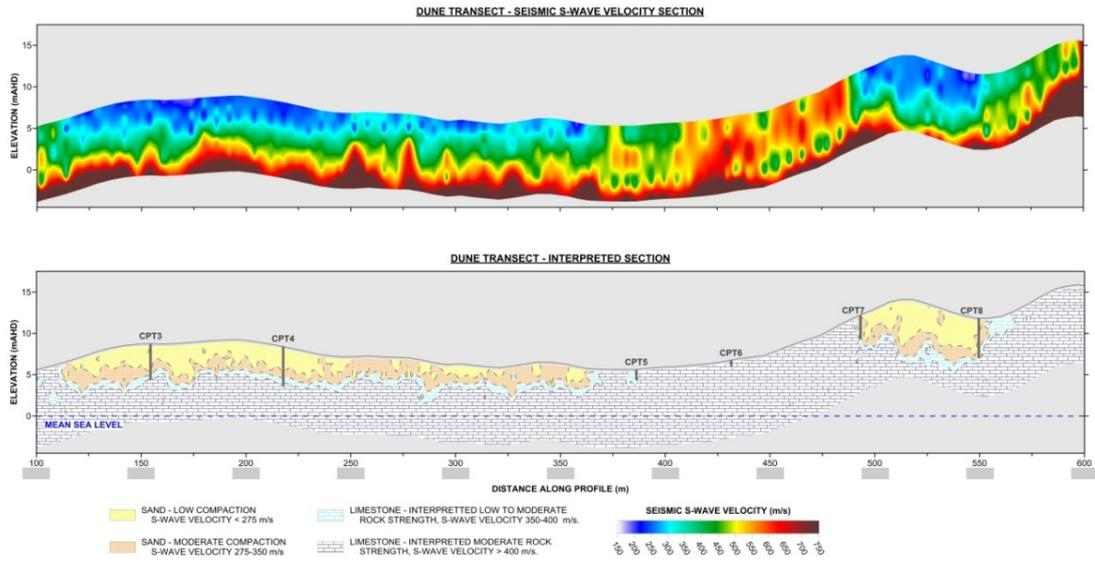
Figure 3. s-wave and interpreted models of dune structure parallel and adjacent to beach with CPT refusal depths overlaid.
