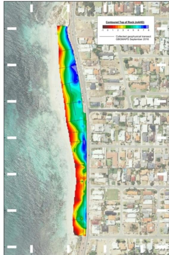
**Figure 4. Contour map showing level (mAHd) to the top of rock along a 600m section of beach foreshore and coastal dune.**
