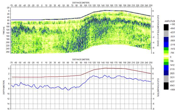
**Figure 1. GPR radar-gram (top) and simplified layer model (bottom) with top of rock level in blue.**
