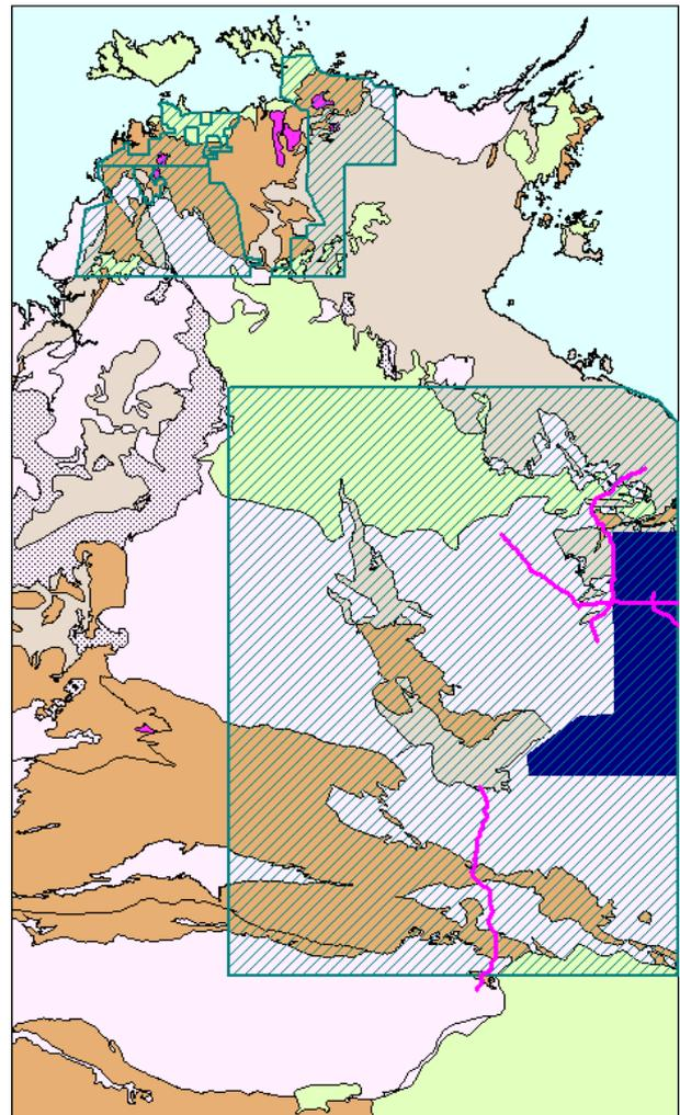
Figure 3. GA-led AEM surveys (green hatching), ground gravity (blue polygons) and deep crustal seismic (pink lines) acquired under the OESP and EFTF programs overlain on the regional geology of the Northern Territory.
