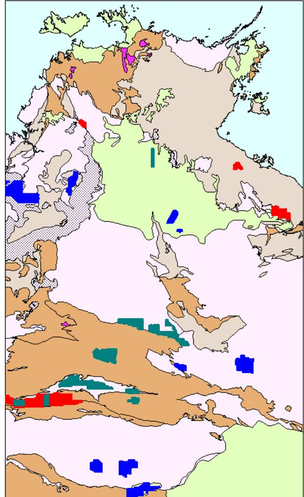
**Figure 1. Industry-led airborne magnetic and radiometric surveys (red polygons), ground gravity (blue polygons) and airborne electromagnetic surveys (green polygons) acquired under the GDC program overlain on the regional geology of the Northern Territory.**
