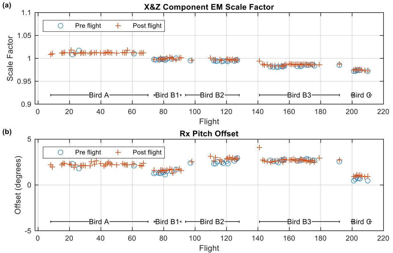
**Figure 4. Summary of the (a) EM scaling factor and (b) receiver pitch offset calibration values that were estimated by our inversion algorithm for each high altitude zero-line over the duration of the survey. The median of each of the five populations (Bird A, B1, B2, B3, and C) are used as the calibration values that are applied to the dataset. Note that many pre-flight zero-lines are not included because they have suspect receiver bird IMU data as noted in the text.**
