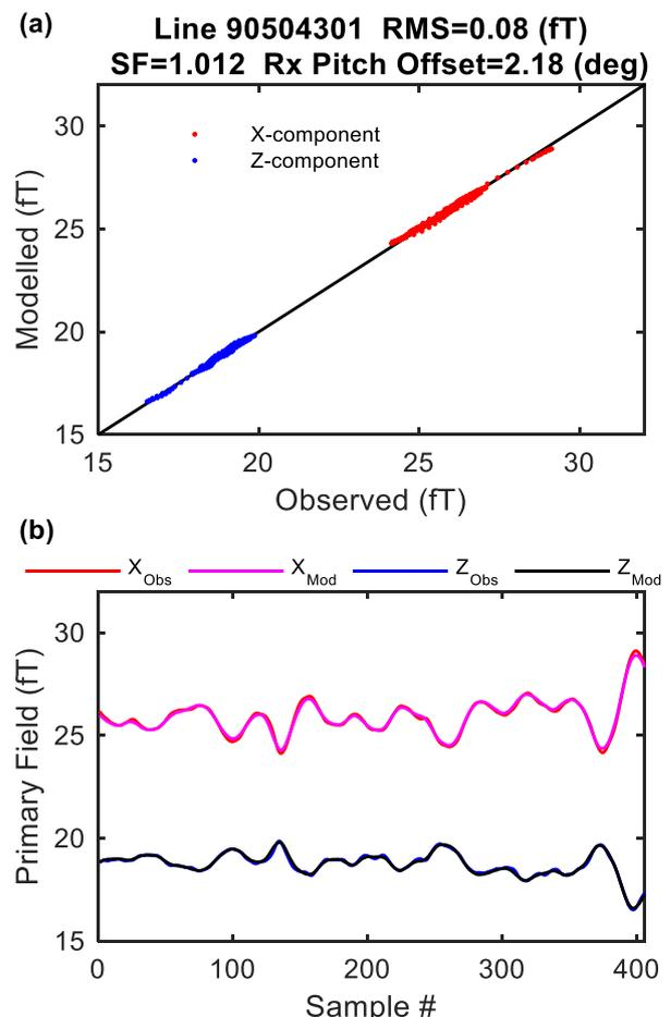
**Figure 3. High altitude zero-line 90504301 after calibration with EM scale factor 1.012 and receiver pitch offset 2.18 degrees. It shows improved agreement between the observed and modelled data in (a) cross-plot and (b) profile form.**
