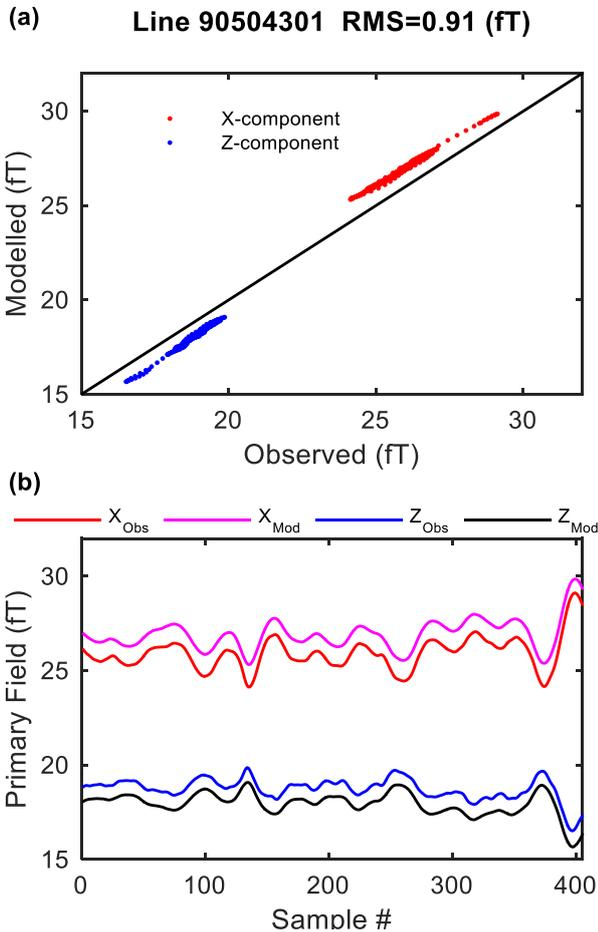
**Figure 2. A preliminary version of high altitude zero-line 90504301 showing the discrepancy between the observed and modelled data in (a) cross-plot and (b) profile form.**
