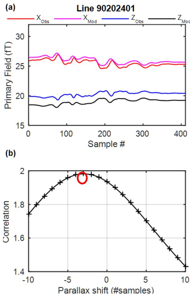
**Figure 1. An early field quality control version of high altitude zero-line 90202401 showing, (a) the observed and theoretically modelled X and Z-component primary field data, and (b) the cross correlation between the observed and modelled data which indicates a three-sample parallax shift.**
