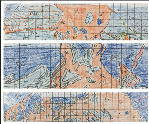
**Figure 4.** Wall mapping from the Nova 2030 OD, East Wall (top) and opposite walls (centre = East, lower = West) of the Nova 2080 OD. The 2030 level shows both examples of the sulphide concentration in  $F_2$  fold hinges with passive and destructive influx. Abbreviations: SXG – mafic granulite, SXQ – mafic granulite gneiss, SM – massive sulphide, SR – sulphide breccia, SS – sulphidic gneiss. Cell size is 1m x 1m.
