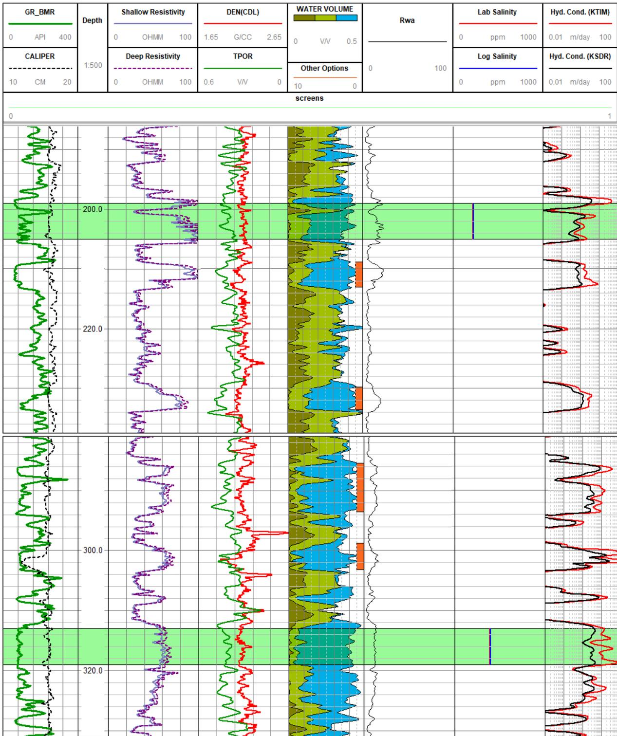
Figure 2. Screen placed over two different aquifers in two bores on the same pad. Other potential aquifers that could be monitored are highlighted with orange bars.
