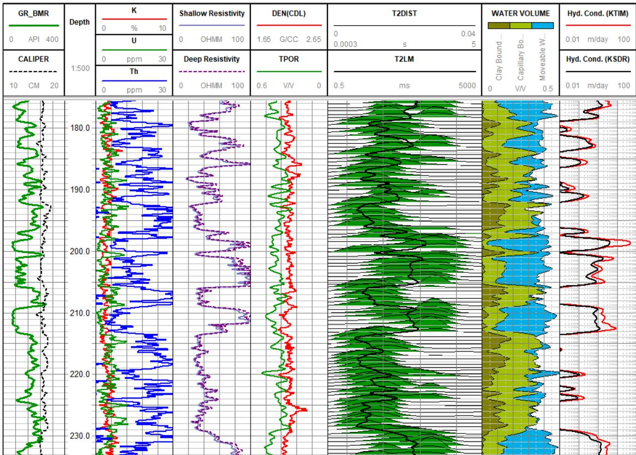
Figure 1. Example BMR log for a monitoring bore installation. Data includes spectral gamma ray, resistivity, density and borehole magnetic resonance. Combined gives both qualitative and quantitative analysis for both short term decisions and long term aquifer analysis
