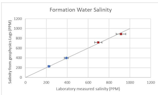
**Figure 3. Cross plot of laboratory and petrophysical log salinity measurements. Data plots very close to the unity line showing great correlation between the data points.**
