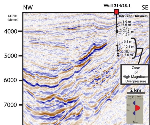
**Figure 1.** Seismic line through Well 214/28-1 located in the Faroe-Shetland Basin, offshore NW Scotland. The seismic line is from a 3D cube acquired 2011-2012 and reprocessed to Pre-Stack Depth Migration in 2016. The lower zone of intrusions, where overpressure was encountered (Figure 5 and 6), extend in a down-dip direction towards a depth of ~6.5 km (21,325 ft).
