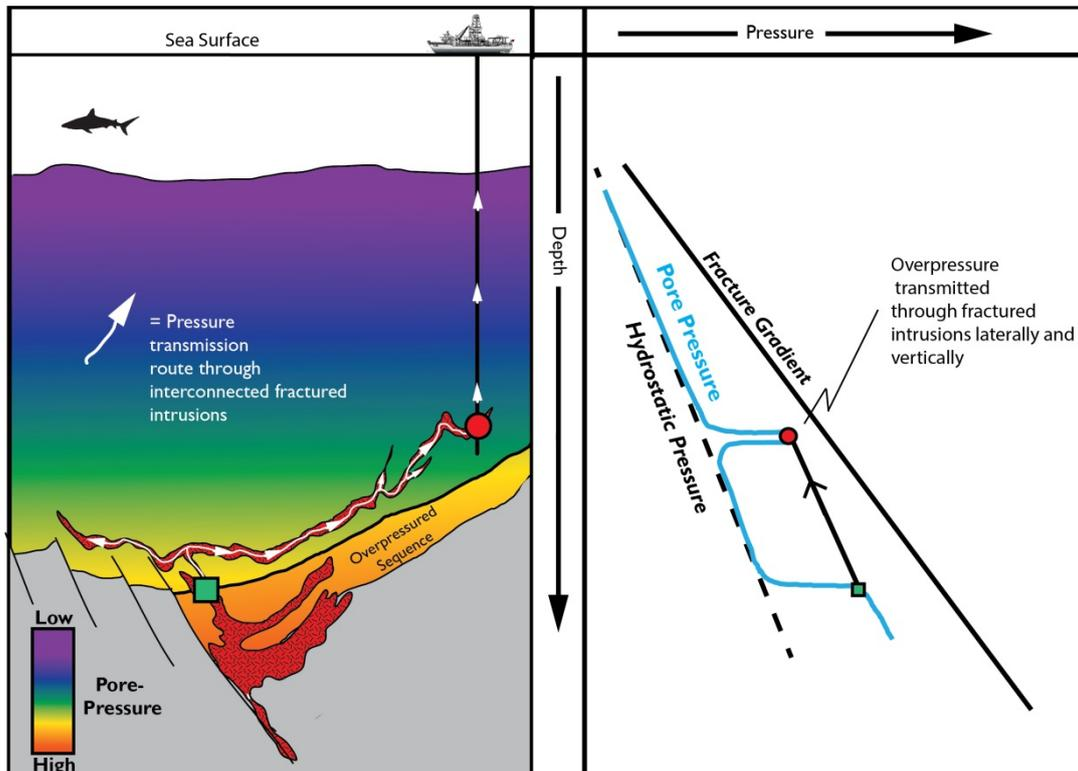
Figure 3. Conceptual diagram showing the principle of pressure transmission through a fractured igneous intrusive complex. Such a process can lead to overpressure being transferred laterally (and vertically) through a basin 10s of km away from its point of origin.
