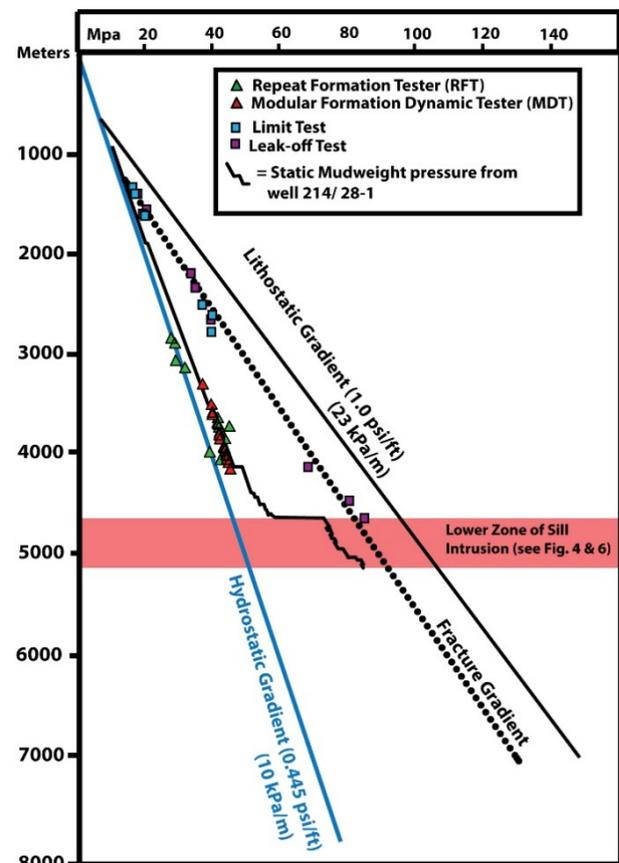
Figure 2. Pressure vs depth plot. Direct pressure data (e.g. RFT) from well 214/28-1 and well 214/27-1 (located 10 km away, that penetrated same stratigraphic succession).
