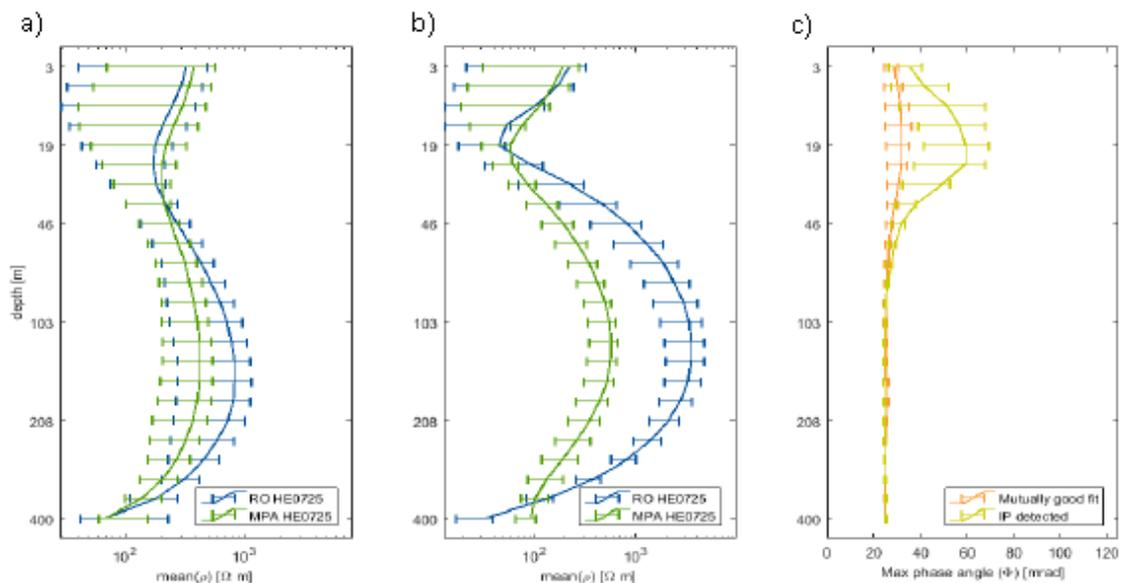
**Figure 2.** a) The depth profiles for resistivity in areas with good fit for both IP (green) and RO (blue) inversion; b) the resistivity profiles for locations with chargeable anomalies ('IP detected'), c) the depth profiles of maximum phase angle with IP inversion, for mutually good fit (orange) and 'IP detected' zones (yellow). 50% confidence intervals are plotted for all estimates.
