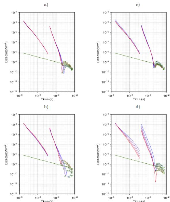
**Figure 1. Four different cases of changes from the basic ‘typical’ IP scenario; a) altering the maximum phase angle of the first and b) second layer, c) altering the resistivity of the first and d) second layer. The negative values are marked with green circles and for clarity are plotted without error bars. A realistic noise level is indicated by the green line.**
