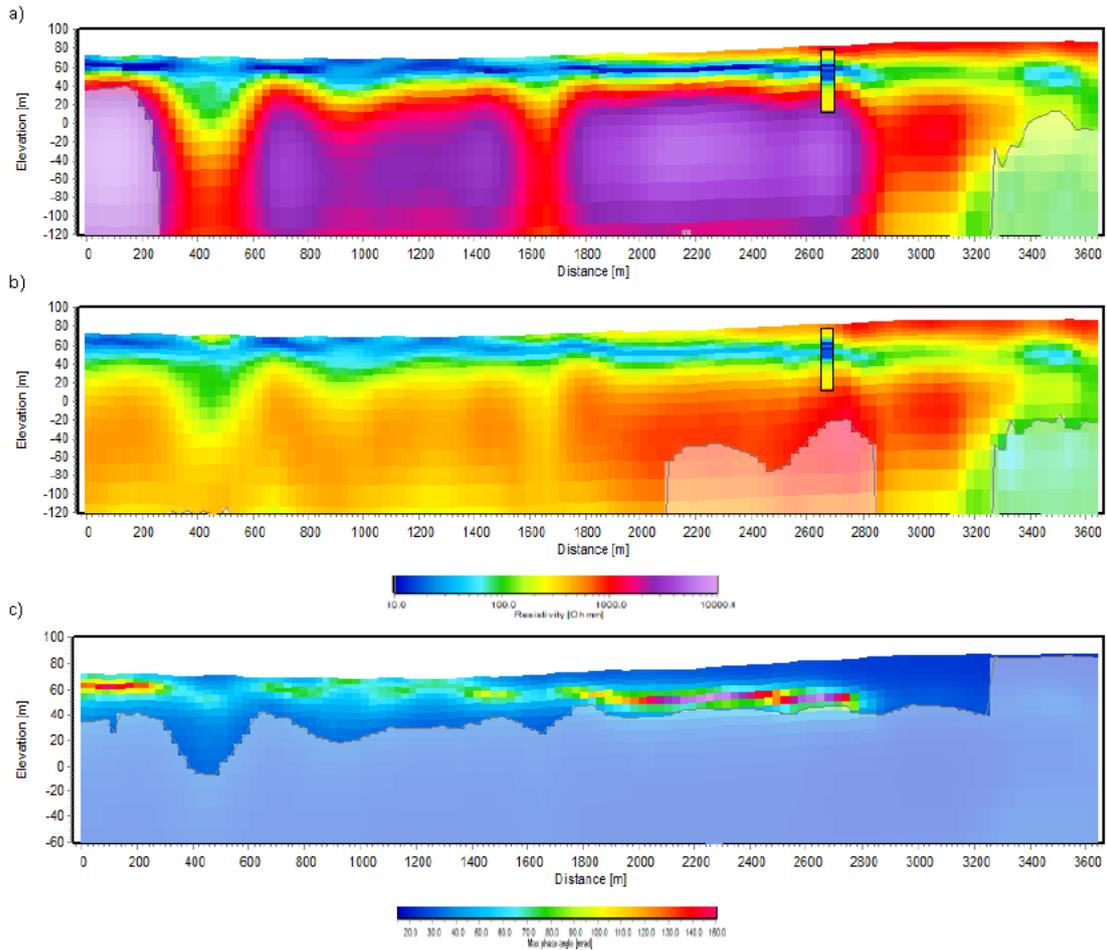
Figure 3. First 3km of the Line 112401. Top panel shows the RO inversion resistivity profile, second panel the MPA resistivity profile, with the well RN 021012. The bottom panel shows the maximum phase angle for the MPA inversion. A borehole with resistivity information is plotted on top.
