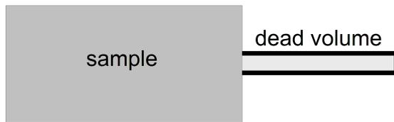
**Figure 2. The arrangement of the fluid-saturated sample and the dead volume surrounded by rigid non-deformable walls.**
