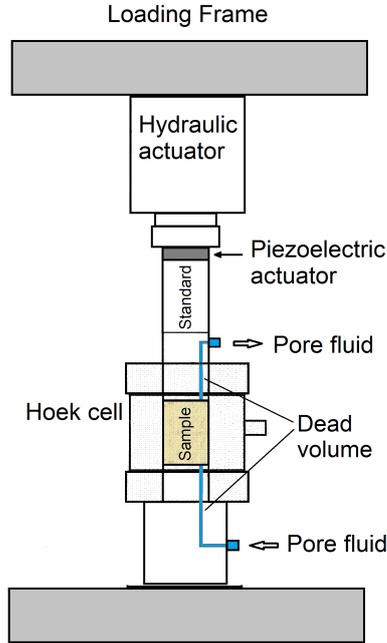
**Figure 1. The mechanical assembly of the low-frequency apparatus based on the forced oscillation method. The minimum allowable dead volume formed by the segments of the pore-fluid lines is highlighted in blue.**
