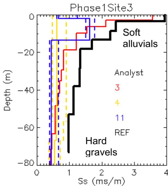
**Figure 1. Site 3, Phase 1. Interpretation of layering from microtremor surface observation with a two-station array. The horizontal axis is shear-wave slowness (inverse of shear-wave velocity). Black: the reference model supplied after all phases of interpretation. Red, yellow, and blue: independent interpretations from three analysts (numbers 3, 4 and 11). Dashed lines are estimates of uncertainty by each analyst. Error estimates were not provided by Analyst 3 for Phase 1 Site 3.**
