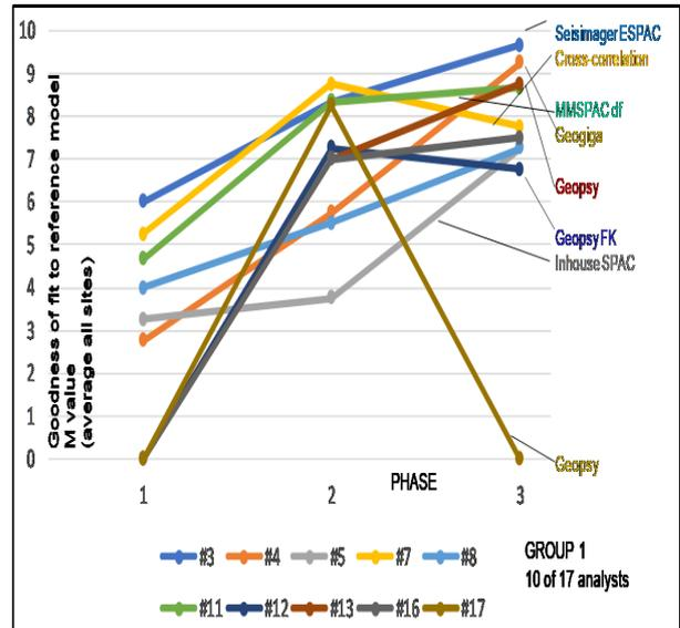
Figure 5. Quality of blind results averaged over all four sites, for the best ten (out of 17) analysts. Software packages used are annotated at right of plot.
