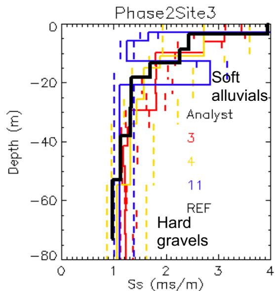
**Figure 2. Site 3, phase 2. Interpretation of layering from microtremor surface observation with a nested pair of three-station triangular arrays. Colours as for Figure 1. Frequency bandwidth achieved with different processing algorithms**
