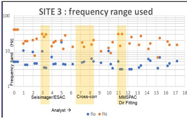
Figure 3. Site 3, Phases 1-3. Blue – minimum frequency. Orange – maximum. Horizontal axis is analyst *n* by number, with Phase 1 plotted at *n.0*, Phase 2 plotted at *n.2*, Phase 3 plotted at *n.4*. The orange bands identify software packages giving the best frequency bandwidth.
