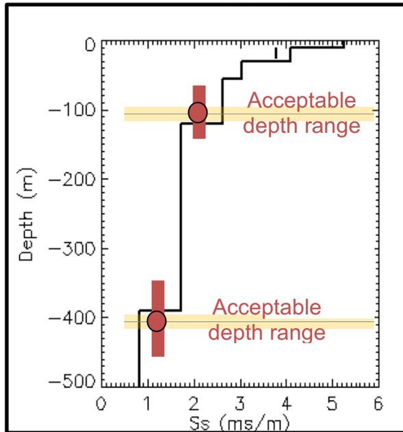
Figure 6. Reference Vs model for site 1, with empirically chosen “acceptable” depth estimate error ranges for an upper interface at 110 m, and lower interface at 407 m.
